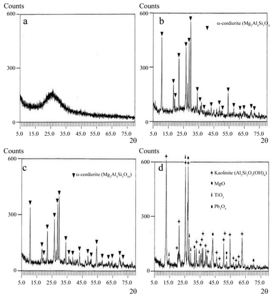
**Fig. 2.** XRD patterns of: (a) the initial glass (fully-amorphous sample), (b) sample 1, (c) sample 2, and (c) powder mixture with the same composition as the parent glass (fully-crystallized sample).
