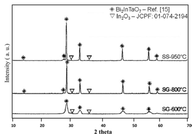
**Fig. 1.** XRD patterns of  $\text{Bi}_2\text{InTaO}_7$  photocatalysts prepared by the sol-gel (SG) and solid state (SS) methods.
