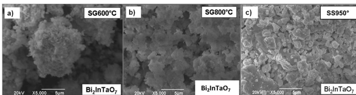
**Fig. 2.** Micrographs of Bi<sub>2</sub>InTaO<sub>7</sub> photocatalysts obtained by the sol-gel and solid state methods. (a) SG-600 °C, (b) SG-800 °C and (c) SS-950 °C.
