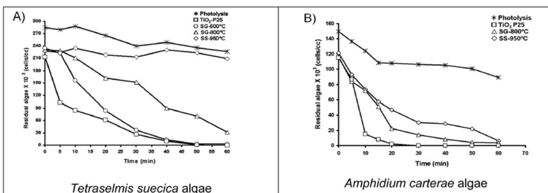
**Fig. 4.** Photocatalytic tests of marine plankton removal using Bi<sub>2</sub>InTaO<sub>7</sub> as photocatalyst under UV-Irradiation. (A) *Tetraselmis suecica* algae (Green tide) and (B) *Amphidium carterae* algae (Red tide)
