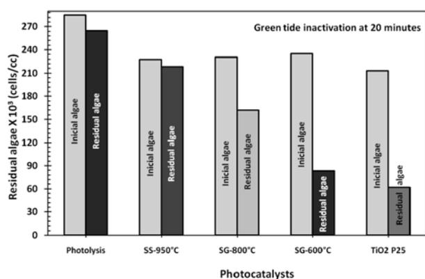
**Fig. 5.** Residual algae measurements after the photocatalytic test after 20 minutes of UV-Irradiation in combination with photocatalysts.
