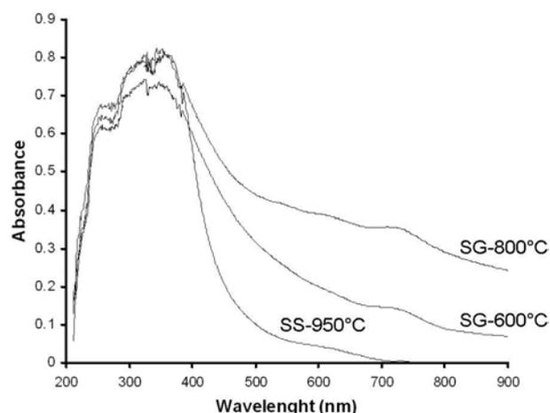
**Fig. 3.** UV-Vis spectra of Bi<sub>2</sub>InTaO<sub>7</sub> photocatalysts prepared by the sol-gel and solid state methods.
