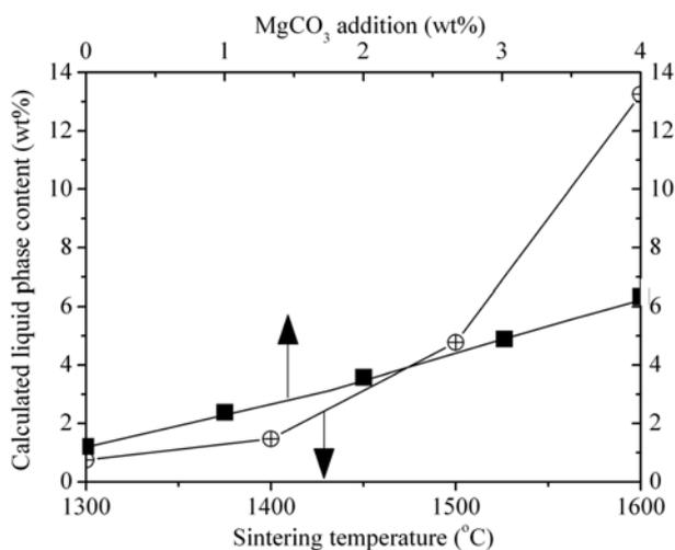
**Fig. 4.** Variations of liquid phase content with  $\text{MgCO}_3$  additions (at  $1500\text{ }^\circ\text{C}$ ) and sintering temperature (containing  $2.93\text{ wt}\%$   $\text{MgCO}_3$ ).
