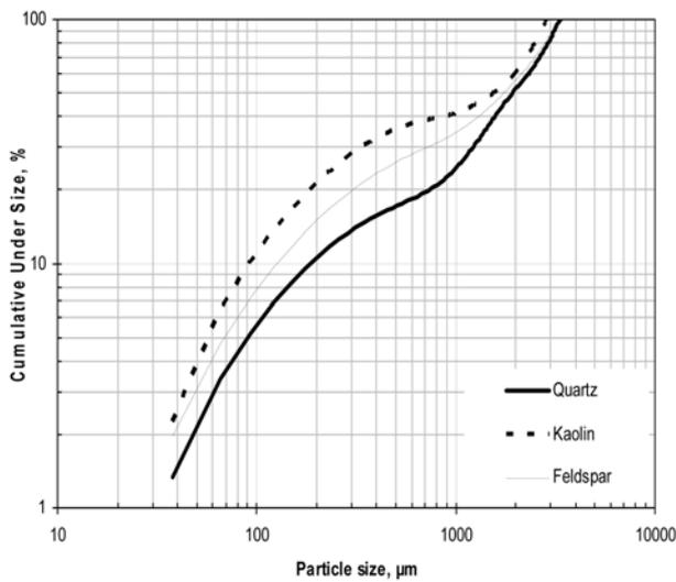
Fig. 1. The cumulative feed size distribution of the raw materials.
