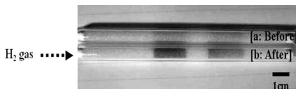
**Fig. 7.** The result of hydrogen-detection: (a) before and (b) after suction inside the pot ground with  $NH_3$ .
