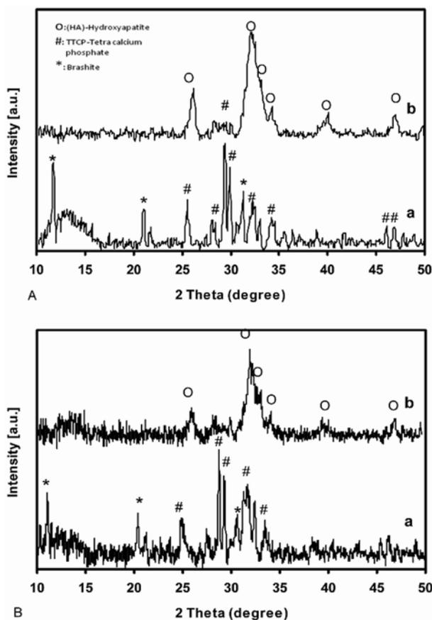
**Fig. 2.** XRD patterns of A) Fiber-free CPC and B) CPC with 15% bioactive glass fiber: a) before soaking in Ringer's solution, b) after soaking in Ringer's solution for 7 days.
