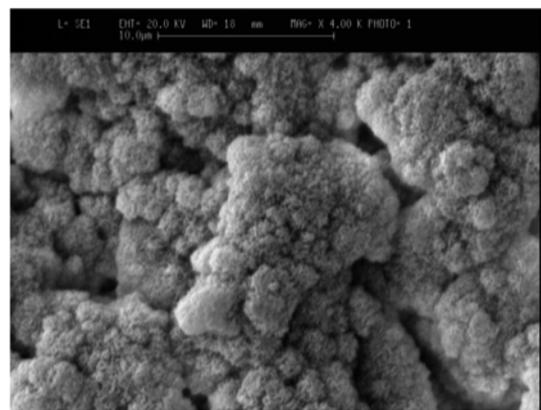
**Fig. 5.** Typical morphology of apatite crystals in the microstructure of a CPC/bioactive glass fiber composite soaked in Ringer's solution for 7 days.
