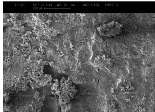
**Fig. 4.** SEM image of a CPC/ bioactive glass fiber composite illustrating pull-out of glass fibers in the CPC matrix.
