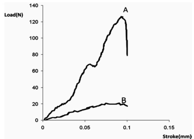
**Fig. 1.** Typical load-displacement curve for: A) bioactive glass-reinforced CPC (15 vol %) and B) unreinforced one.
