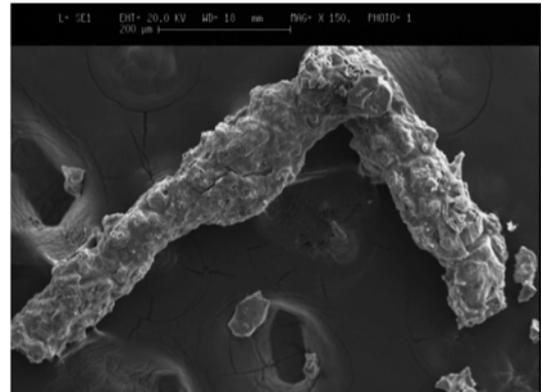
**Fig. 3.** SEM micrograph of a sol gel derived bioglass fiber.
