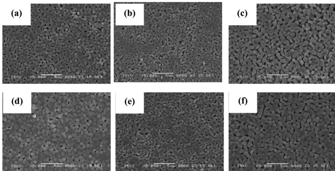
**Fig. 2.** SEM micrograph of BT ceramics sintered at different temperatures (a) BT01 1100 °C (b) BT03 1100 °C (c) BT05 1100 °C (d) BT01 1150 °C (e) BT03 1150 °C (f) BT05 1150 °C.
