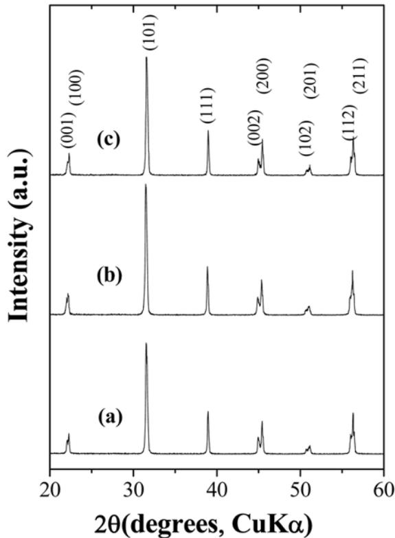
**Fig. 1.** XRD patterns of BT ceramics sintered at 1150 °C for 30 minutes from three types of BT powders (a) BT01 (b) BT03 (c) BT05.
