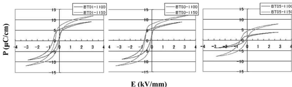
Fig. 4. P-E hysteresis loops of BT ceramics sintered by the microwave sintering method at different temperatures.
