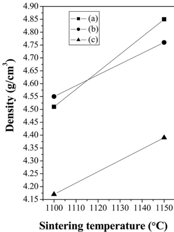
Fig. 3. The density of BT specimens sintered by the microwave sintering method at different temperatures from three types of BT powders (a) BT01 (b) BT03 (c) BT05.
