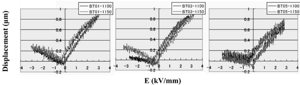
Fig. 5. The displacement versus electric field for BT ceramic sintered by the microwave sintering method at different temperatures.
