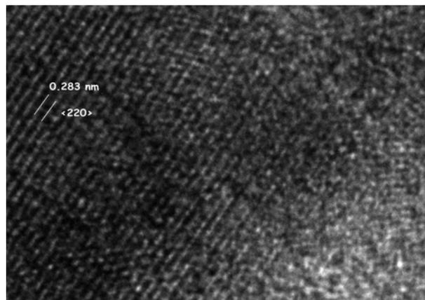
**Fig. 6.** TEM micrograph of  $\text{CuAl}_2\text{O}_4$  powder synthesized at  $800^\circ\text{C}$  with  $R = 4$ .
