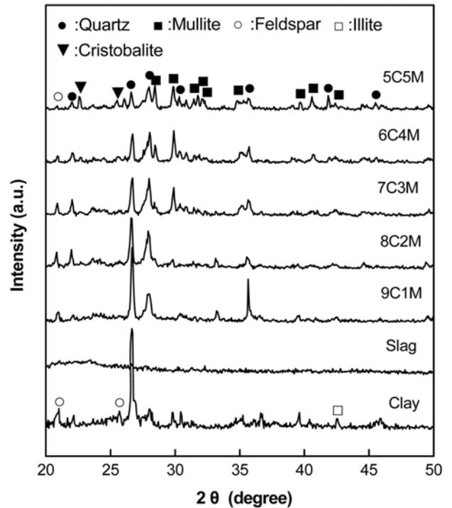
Fig. 2. XRD analysis of raw materials and brick specimens with MIR slag contents fired at 1000 °C for 2 h.
