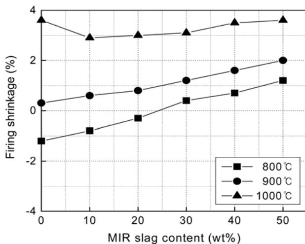
Fig. 4. Firing shrinkages of the brick specimens as a function of the MIR slag content and firing temperature.
