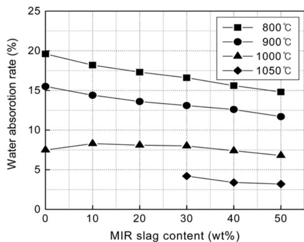
Fig. 6. Water absorption rates of the brick specimens as a function of the MIR slag content and firing temperature.
