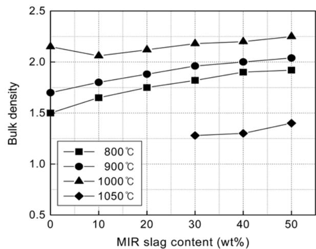
Fig. 5. Bulk densities of brick specimens as a function of the MIR slag content and firing temperature.
