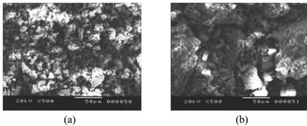
**Fig. 1.** SEM images of clay (a) and MIR slag (b).
