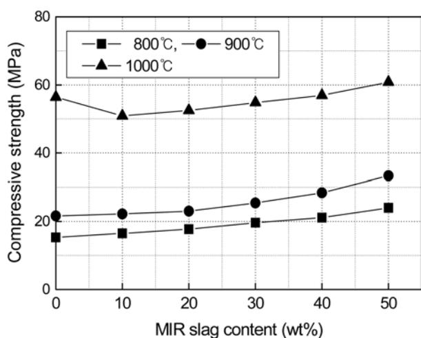
Fig. 7. Compressive strengths of the brick specimens as a function of the MIR slag content and firing temperature.
