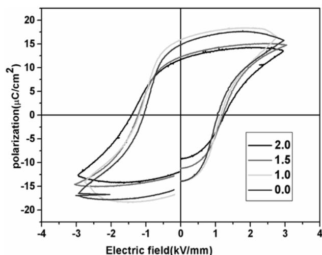
Fig. 6. The P-E hysteresis loops of the  $K_{0.5}Na_{0.5}NbO_3$  ceramics as a function of x mol% ZnO.
