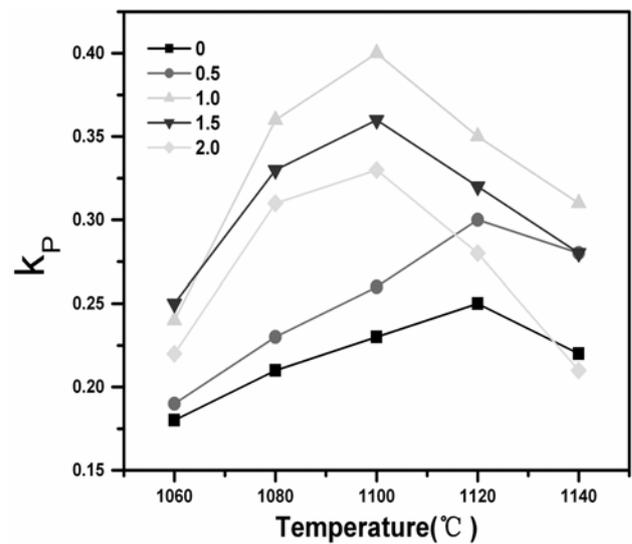
**Fig. 5.**  $k_p$  of the  $K_{0.5}Na_{0.5}NbO_3$  ceramics as a function of  $x$ mol% ZnO.
