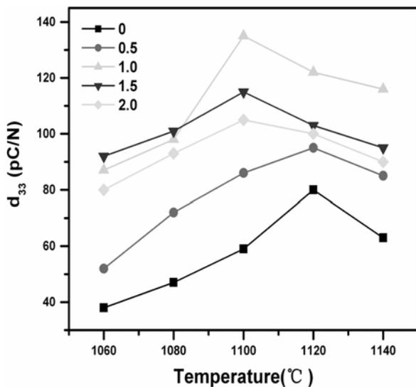
**Fig. 4.**  $d_{33}$  of the  $K_{0.5}Na_{0.5}NbO_3$  ceramics as a function of  $x$ mol% ZnO.
