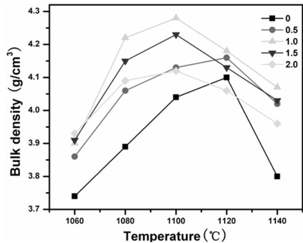
Fig. 2. Bulk densities of the  $K_{0.5}Na_{0.5}NbO_3$  ceramics as a function of x mol% ZnO.
