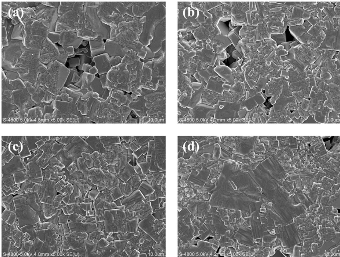
**Fig. 3.** SEM images of the  $K_{0.5}Na_{0.5}NbO_3$  ceramics with  $x$ mol% ZnO sintered at  $1100^\circ\text{C}$  for 1h (a)  $x = 0$ ; (b)  $x = 0.5$ ; (c)  $x = 1.0$ ; (d)  $x = 2.0$ .
