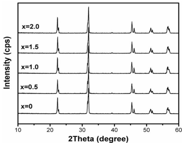
Fig. 1. XRD patterns of the  $K_{0.5}Na_{0.5}NbO_3$  ceramics as a function of x mol% ZnO sintered at 1100 °C for 1 h.
