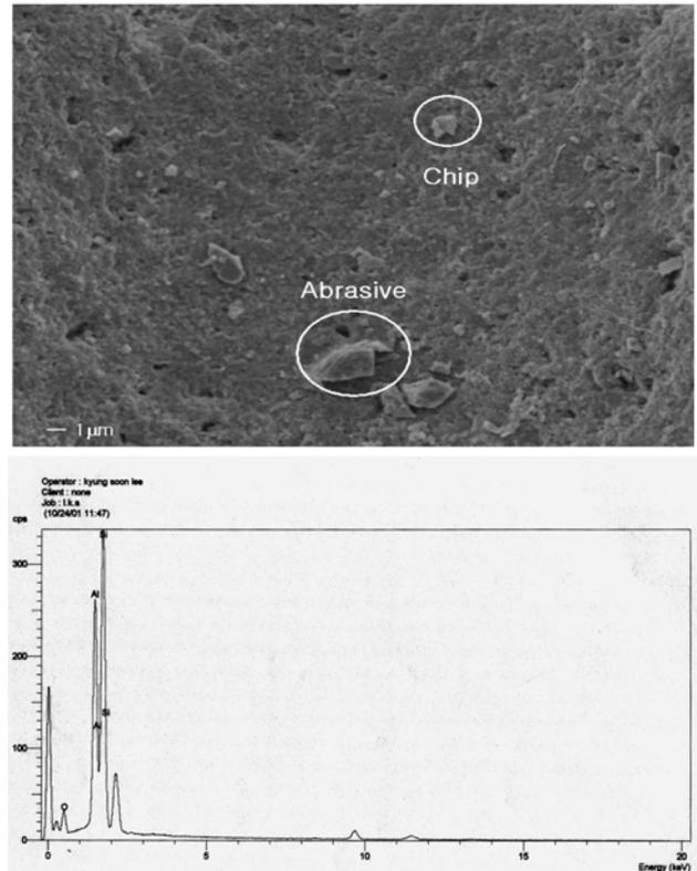
Fig. 8. SEM images and EDX spectrum of an abrasive particle and chip.
