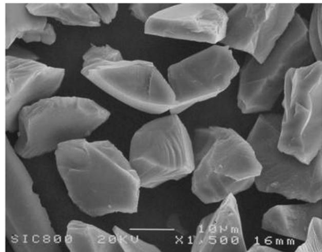
(b) SiC #800 (14 $\mu$ m)
