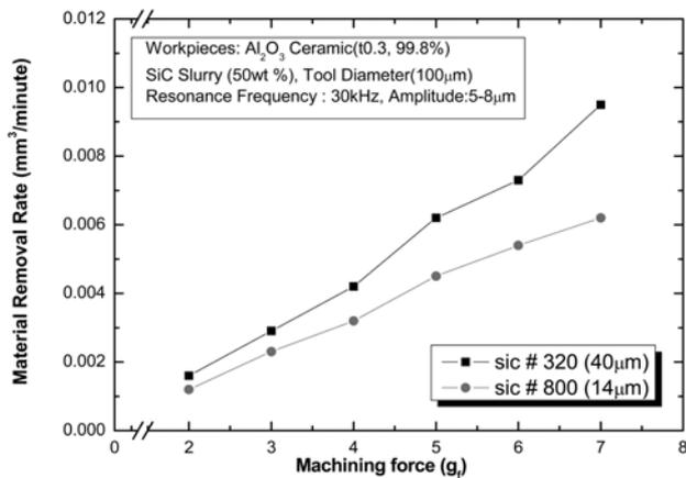
Fig. 7. Relation between machining force and MRR.
