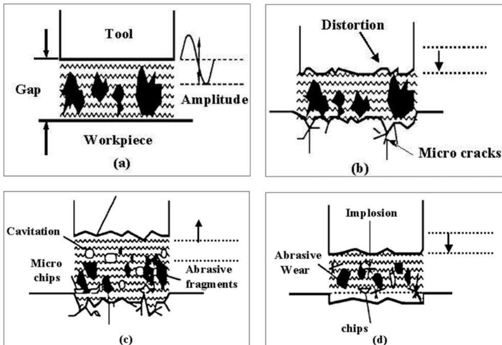
Fig. 2. Material removal mechanism.
