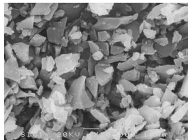
(c) SiC #8000 (1 $\mu$ m)**Fig. 4.** SEM images of the abrasive particles.
