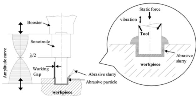
Fig. 1. Schematic diagram of ultrasonic machining.
