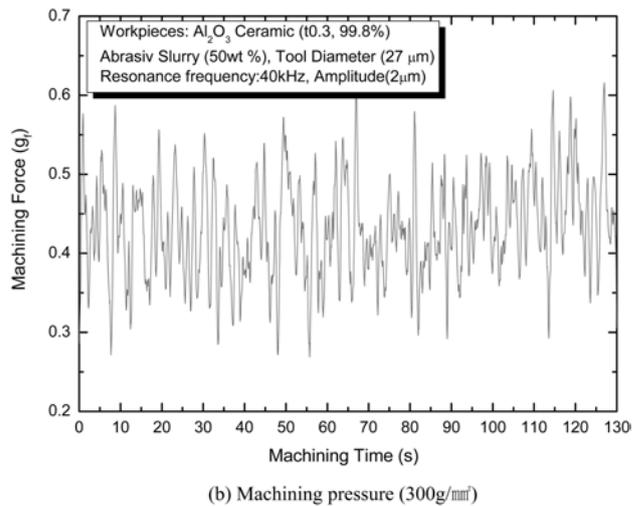
(b) Machining pressure (300g/mm<sup>2</sup>)
