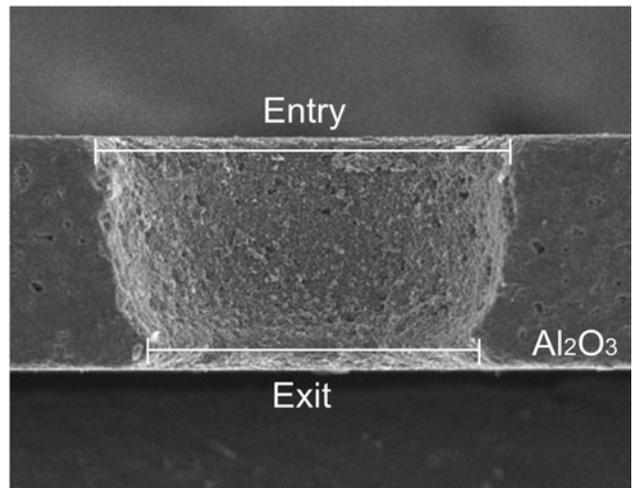
(b) Cross section of a micro-hole
