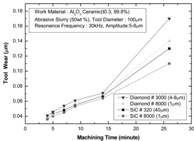
Fig. 10. Influence of different abrasive grit sizes on tool wear.
