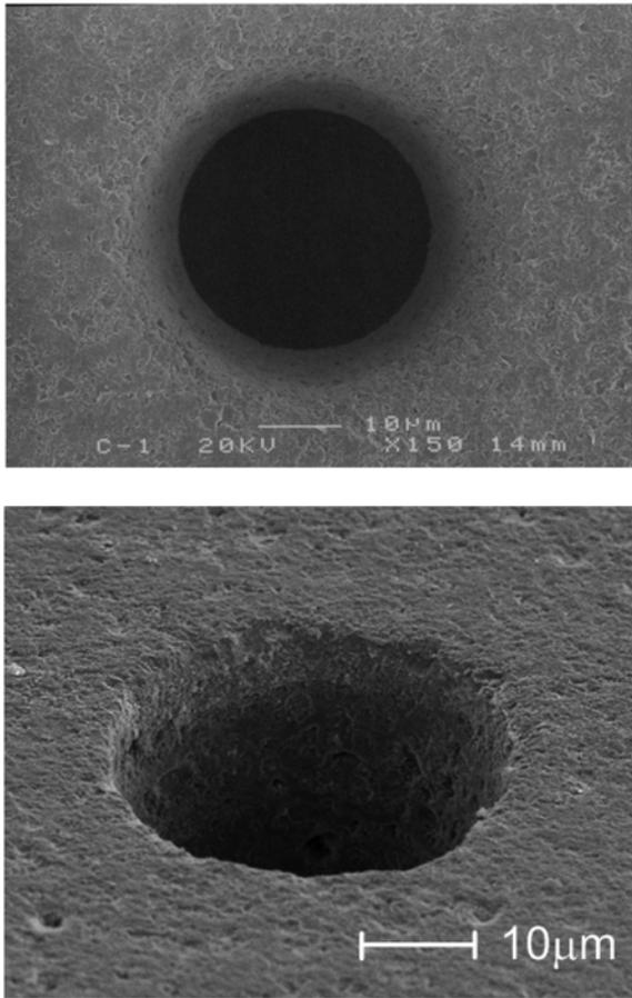
**Fig. 12.** Micro-hole made by USM in  $Al_2O_3$  ceramics (SiC#8000, 50wt.%, depth: 300  $\mu m$ , aspect ratio: 10).
