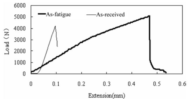
**Fig. 9.** Relation between load and extension of 3D-C/SiC bolts after a tensile test and a fatigue tensile test at room temperature.
