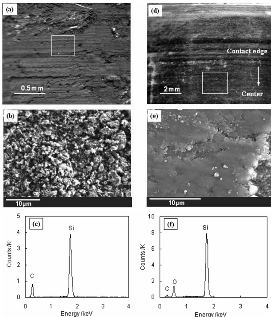
**Fig. 8.** SEM microstructure and EDS analysis of the worn surfaces of the C/SiC hinge bearing tested at room temperature in air (as shown in (a)-(c)) and at high temperatures in a combustion environment (as shown in (d)-(f)).
