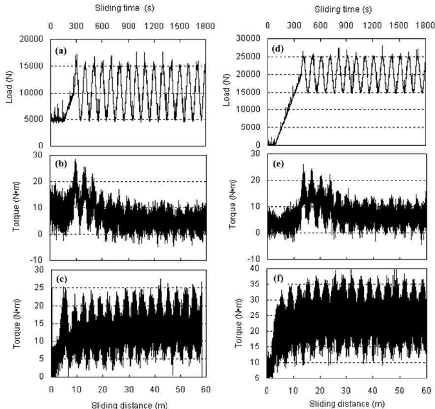
**Fig. 7.** The relationship of friction torque versus sliding time of the C/SiC composites axle under a cyclic loading condition at a gas-temperature of 1800 °C in a combustion environment, comparing with that at room temperature. (a) 5~15 kN loading condition, (b) torque at room temperature in air, (c) torque in a combustion environment, (d) 15~25 kN loading condition, (e) torque at room temperature in air, (f) torque in a combustion environment.
