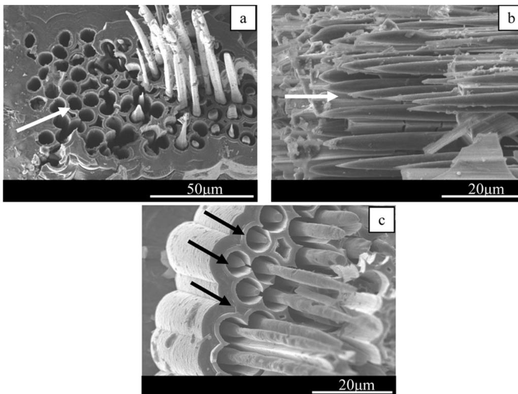
**Fig. 5.** The morphology of oxidized fibers on fracture surfaces of C/SiC composites tested at 1800 °C in a combustion environment (the direction of the heat flux is marked by an arrow).
