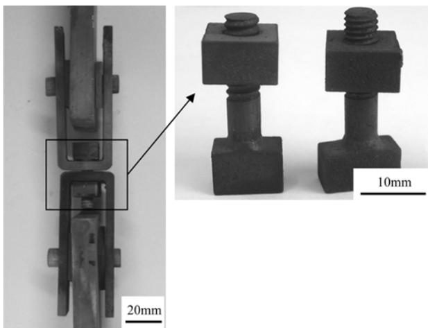
**Fig. 3.** Clamping fixture for tensile tests of 3D needed C/SiC bolts at high temperatures in combustion environments.
