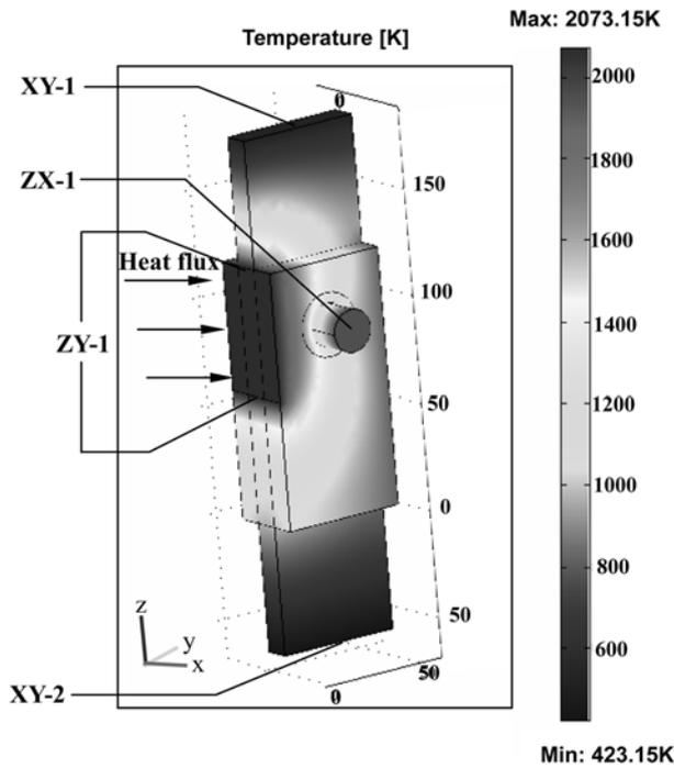
**Fig. 6.** Temperature distribution in a C/SiC composite hinge bearing when tested at a gas-temperature of 1800 °C in a combustion environment.
