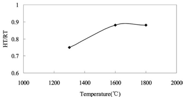
**Fig. 11.** Relationship between strength conversation rates of 3D-C/SiC bolts and test temperature in a combustion environment.
