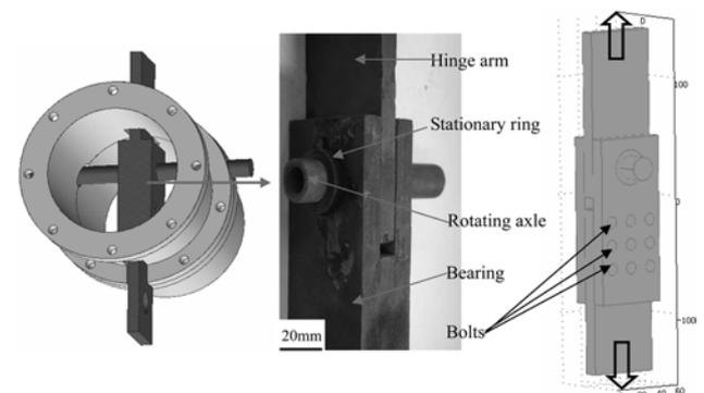
**Fig. 2.** Test schematic of friction behavior of C/SiC composites hinge bearing sample in high temperature combustion environment.
