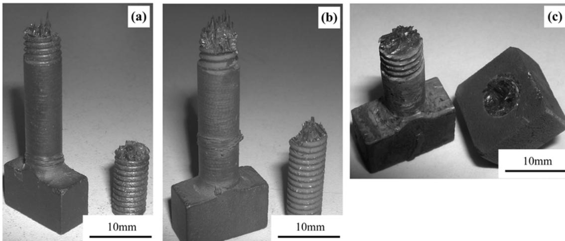
**Fig. 10.** The fractured 3D needed C/SiC bolts (a) after a tensile test at R.T., (b) after a fatigue tensile test at R.T., (c) after a tensile test at 1800 °C in a combustion environment.
