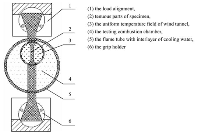
**Fig. 1.** Schematic diagram of the stress-oxidation tests and tensile tests of C/SiC composites in high temperature combustion environment.
