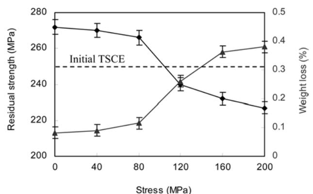
**Fig. 4.** The residual strength and weight loss of C/SiC composites after exposure for 10 minutes at 1500 °C under different applied stresses in a combustion environment.
