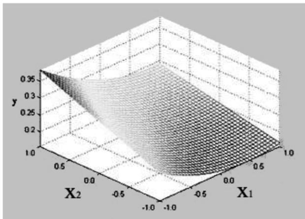
**Fig. 9.** Response surface model for  $Al_2O_3$  particle size ( $x_1$ ) and amplitude of cyclic compaction pressure ( $x_2$ ) in the case of friction coefficient  $x_3 = 0$ .
