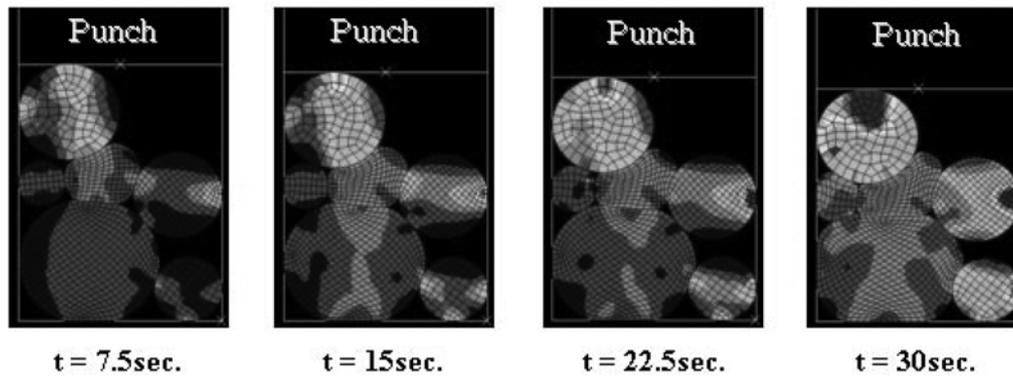
Fig. 4. Formed shapes and principal stresses of 6 particles during the powder compaction.
