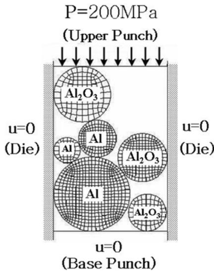
**Fig. 2.** Finite element modeling of ceramic powders and boundary conditions for simulating the powder compaction process.
