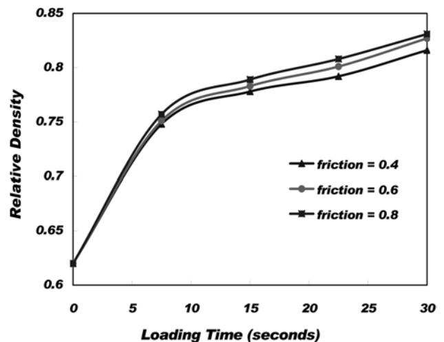
Fig. 6. Comparison of relative density among friction coefficients 0.4, 0.6, and 0.8.
