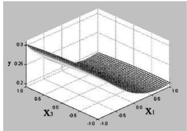
**Fig. 10.** Response surface model for  $Al_2O_3$  particle size ( $x_1$ ) and coefficient of friction ( $x_3$ ) in the case of cyclic compaction pressure amplitude  $x_2 = 0$ .
