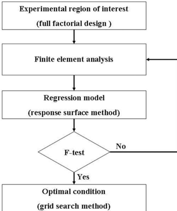
Fig. 7. Schematic flow for optimizing process parameters of powder compaction.
