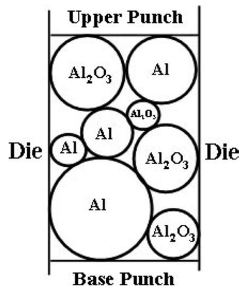
Fig. 1. 2-dimensional view of powder compaction device and ceramic powders.
