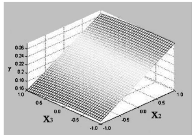
**Fig. 11.** Response surface model for amplitude of cyclic compaction pressure ( $x_2$ ) and coefficient of friction ( $x_3$ ) in the case of particle size  $x_1 = 0$ .
