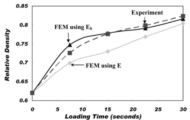
Fig. 5. Comparison of relative densities obtained from FEM analyses and experiment during the powder compaction.
