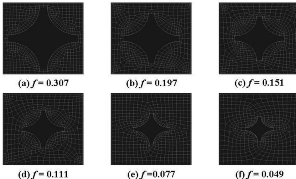
**Fig. 3.** Cross pore-solid models for calculating homogenized elastic modulus associated with porosities(f).
