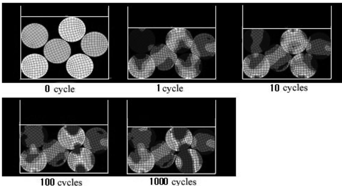
Fig. 8. Formed shapes and principal stresses associated with pressure cycles in the case of  $x_1 = x_2 = x_3 = 0$ .
