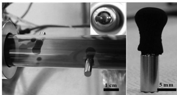
**Fig. 2.** MWNTs collection using an electromagnet.
