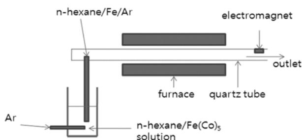
**Fig. 1.** A schematic of the pyrolysis apparatus.
