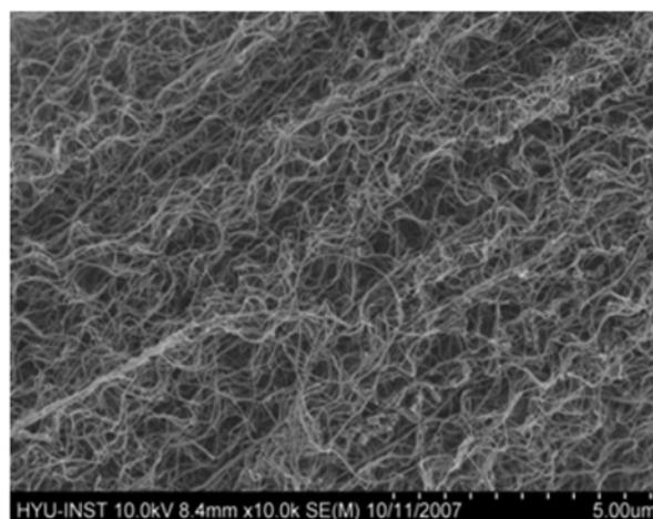
**Fig. 3.** SEM image of the as-synthesized carbon material produced by catalytic reaction of n-hexane over Fe catalyst at 950 °C.
