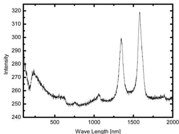
**Fig. 5.** Raman spectrum of the MWCNTs synthesized at 950 °C.
