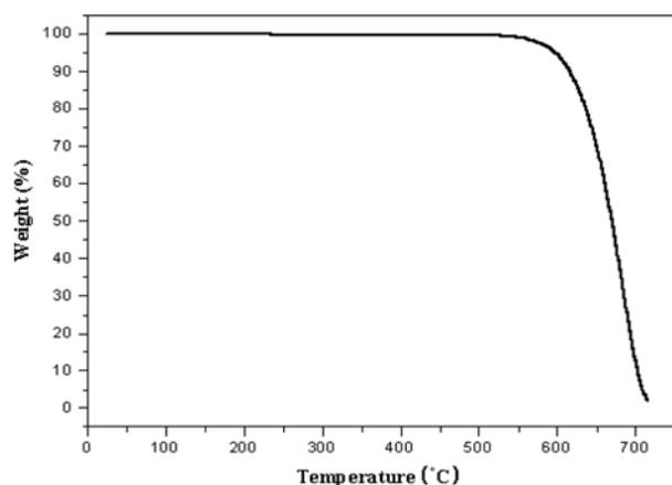
**Fig. 4.** TGA output of MWNTs after the mechanical purification. Fe catalyst particles have been almost completely removed (over 95%) after mechanical purification using a high vacuum ( $1.3 \times 10^{-10}$  MPa) and a high temperature  $\sim 1500$  °C).
