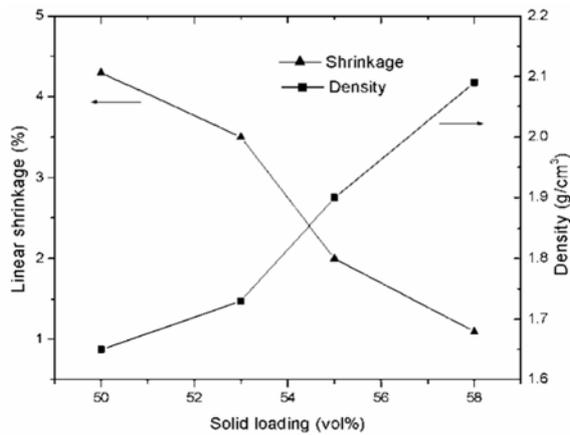
Fig. 3. Effects of solid loading on linear drying shrinkage and green density.
