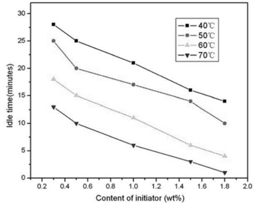
**Fig. 2.** Idle time as a function of initiator content and gelling temperature.
