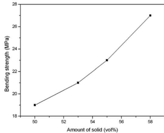
Fig. 5. Effects of solid loading on green strength.
