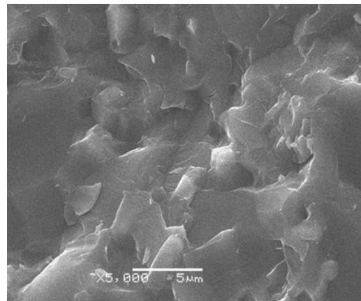
Fig. 10. SEM micrographs of fracture of RBSC obtained by gelcasting.
