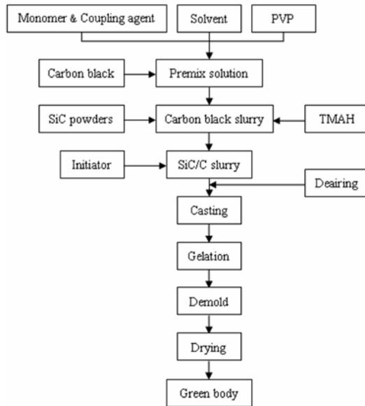
**Fig. 1.** Flowchart of gelcasting process.
