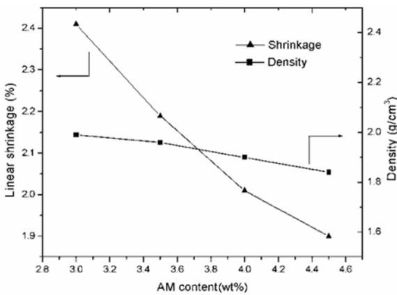
Fig. 4. Effects of monomer content on linear drying shrinkage and green density.
