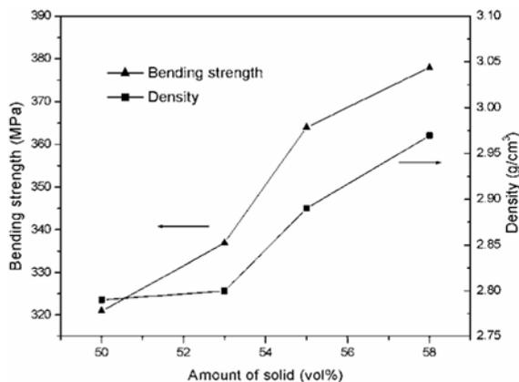
Fig. 8. Flexural strength and bulk density of sintered bodies versus solids loading.
