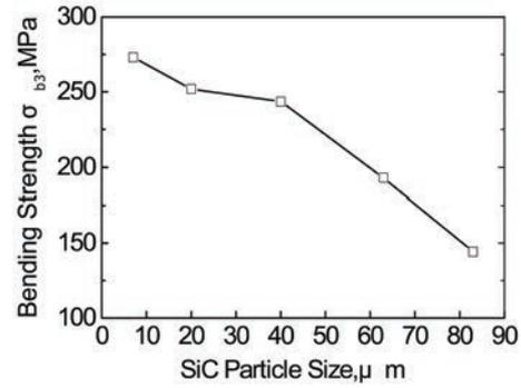
**Fig. 3.** Influence of particle size on bending strength of SiC/Al.
