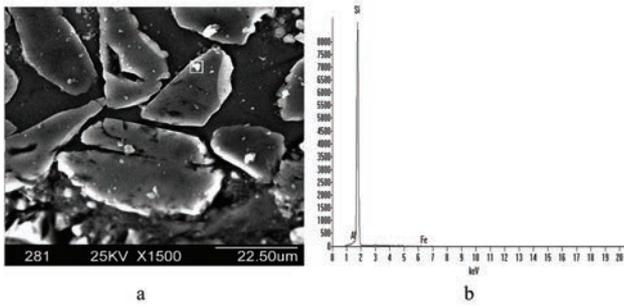
**Fig. 2.** Small white products ( □ ) on the SiC surface, a) metallographic surface (sample 3); b) chemical composition at ‘ □ ’ by EDX.
