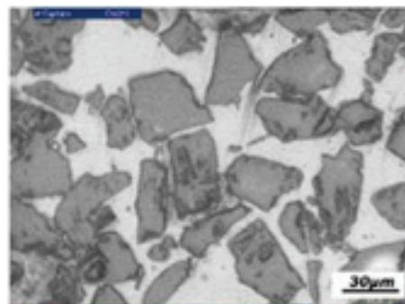
**Fig. 1.** Microstructure of the SiC/Al composite (sample 3).
