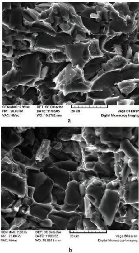
**Fig. 6.** Fractograph of the composites: a) sample 2-2; b) sample 2-1.
