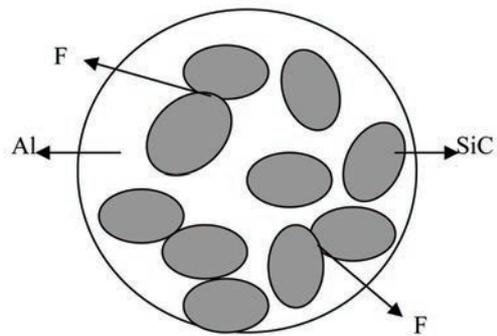
**Fig. 5.** Schematic showing the microstructural model of SiC/Al composite.
