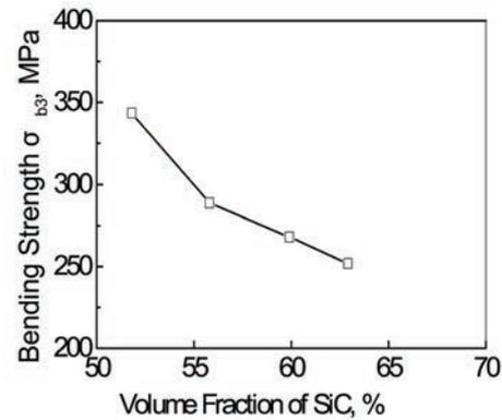
**Fig. 4.** Influence of volume fraction of SiC on bending strength of SiC/Al.
