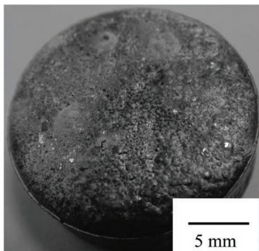
Fig. 2. Macrograph of  $AgSnO_2$  material sintered at  $700^\circ C$  for 4 h.
