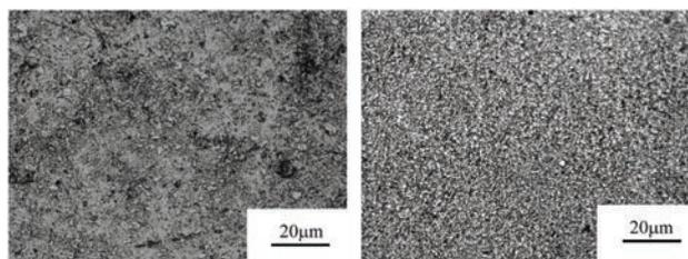
Fig. 3. Microstructure of  $AgSnO_2$  and  $AgSnO_2-Y_2O_3$  materials sintered at  $700^\circ C$  and held for 4 h. (a)  $AgSnO_2$  material, (b)  $AgSnO_2-Y_2O_3$  material
