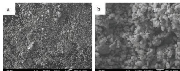
**Fig. 1.** SEM micrographs of  $AgSnO_2$  compound powder milled for 60 h at low and high magnification. (a) low magnification (b) high magnification.
