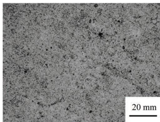
Fig. 4. Microstructure of  $AgSnO_2-Y_2O_3$  material after repressing at 300 MPa and resintering at  $700^\circ C$  for 1 h.
