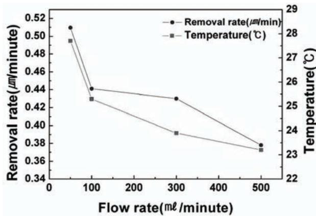
Fig. 4. Changes of removal rate and temperature in the exit-point according to the slurry flow rate.
