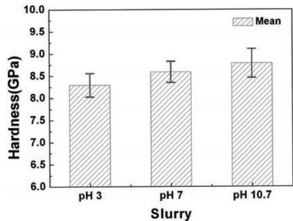
Fig. 6. Hardness variation with slurries.
