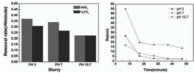
Fig. 2. (a) Removal rate according to the slurry pH, H<sub>3</sub>PO<sub>4</sub> and HNO<sub>3</sub>. (b) Roughness of surface according to pH 3, 7, 10.7 as a function of time.
