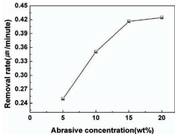
Fig. 3. Change of removal rate according to the abrasive concentration.
