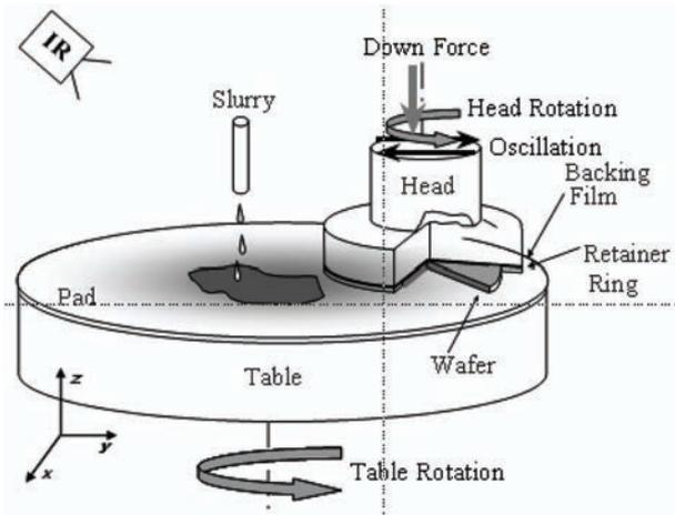
Fig. 1. Schematic of CMP system.
