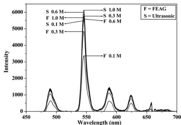
**Fig. 8.** Photoluminescence spectra of the LaPO<sub>4</sub>:Tb phosphor powders prepared by the FEAG and ultrasonic spray pyrolysis processes.
