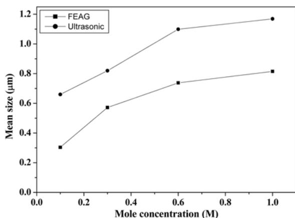
Fig. 3. Mean sizes of the as-prepared powders obtained by the FEAG and ultrasonic spray pyrolysis processes.
