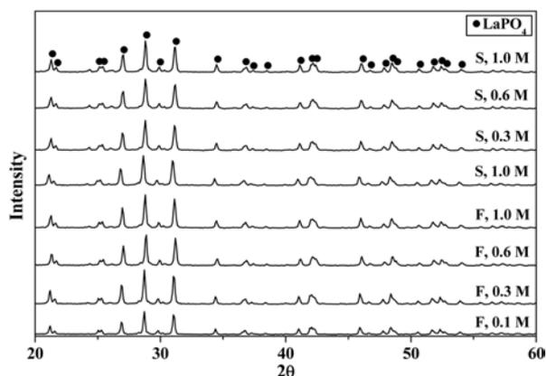
**Fig. 7.** XRD patterns of the LaPO<sub>4</sub>:Tb phosphor powders prepared by the FEAG and ultrasonic spray pyrolysis processes after post-treatment at 1050 °C (S: Ultrasonic, F: FEAG).
