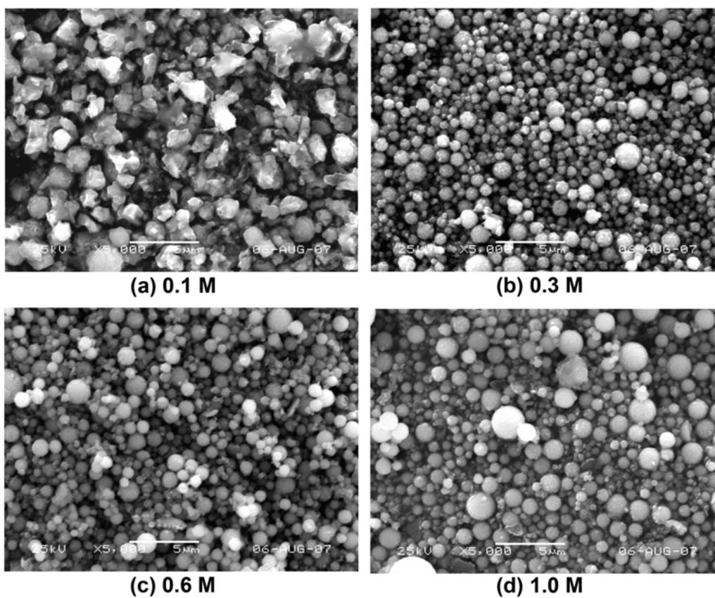
Fig. 5. SEM images of the post-treated  $\text{LaPO}_4:\text{Tb}$  phosphor powders obtained by the FEAG process.
