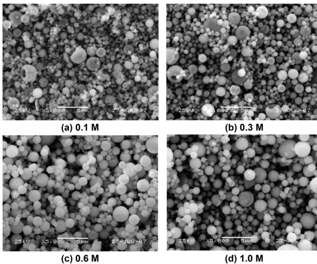
Fig. 6. SEM images of the post-treated  $\text{LaPO}_4:\text{Tb}$  phosphor powders obtained by the ultrasonic spray pyrolysis.
