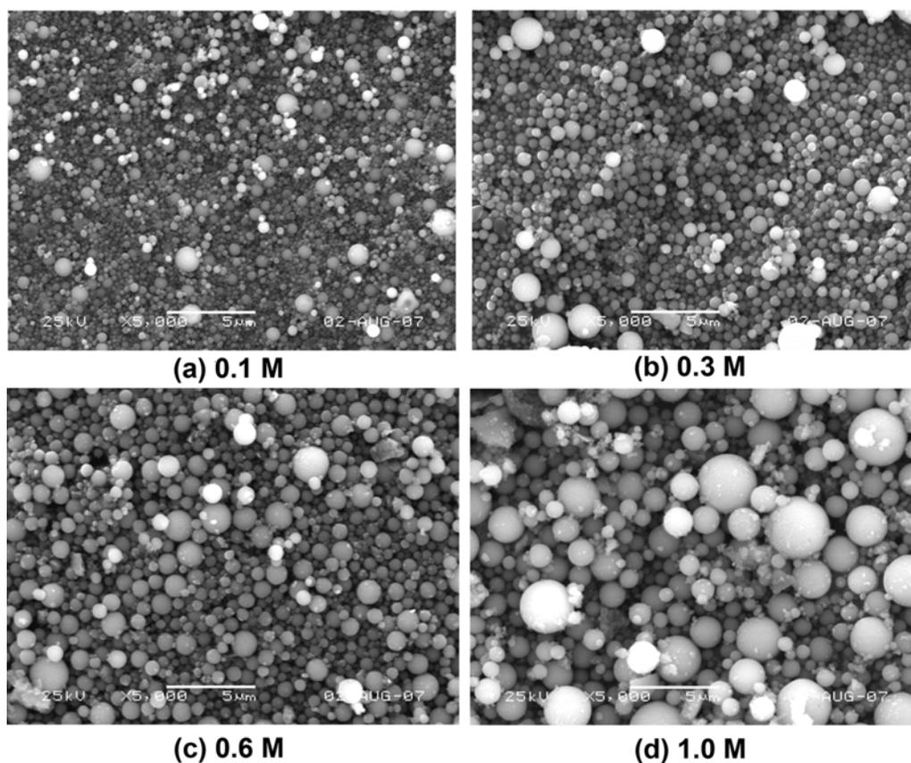
Fig. 1. SEM images of the as-prepared powders obtained by the FEAG process.
