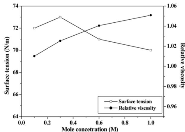
Fig. 4. Surface tensions and relative viscosities of the spray solutions at different concentrations.
