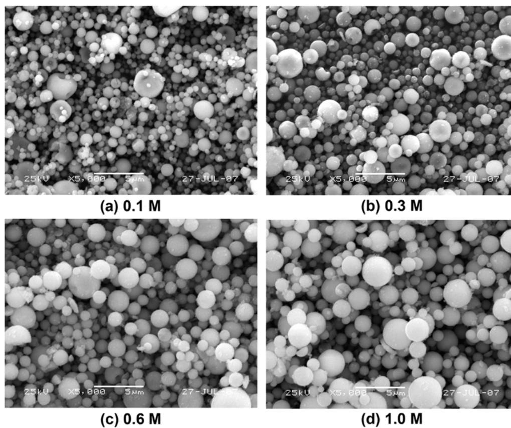
Fig. 2. SEM images of the as-prepared powders obtained by the ultrasonic spray pyrolysis.
