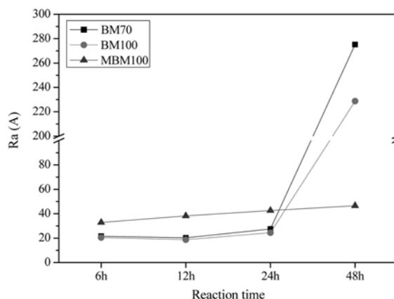
**Fig. 4.** Surface roughness of coating films as a function of reaction time.
