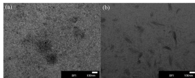
**Fig. 1.** TEM images of boehmite sol powders. (a) spherically shaped boehmite (b) fibrous shaped boehmite.
