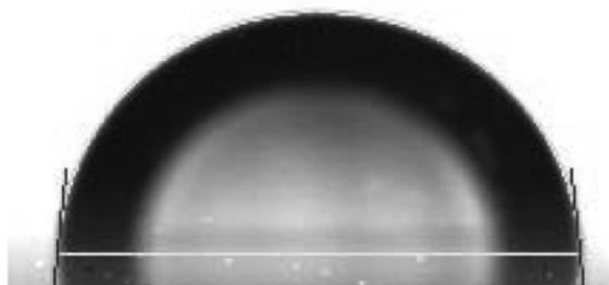
**Fig. 3.** Typical drop of water on a coating film (specimen MBM100 reacted for 12 h) for measuring contact angle. The amount of water dropped on a coating film was 10 µl.
