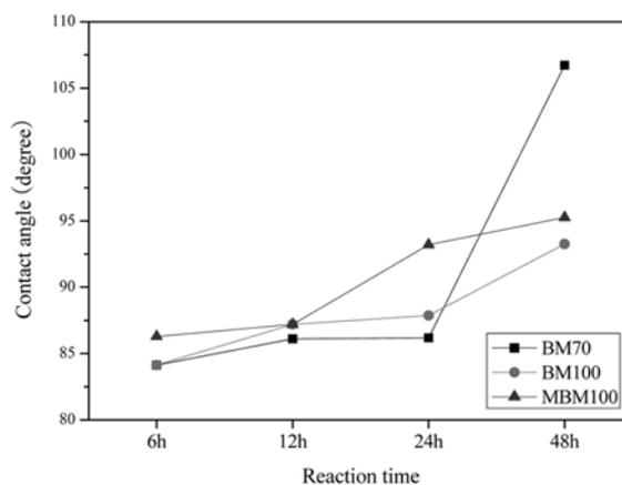
**Fig. 2.** Contact angle of coating films as a function of reaction time.
