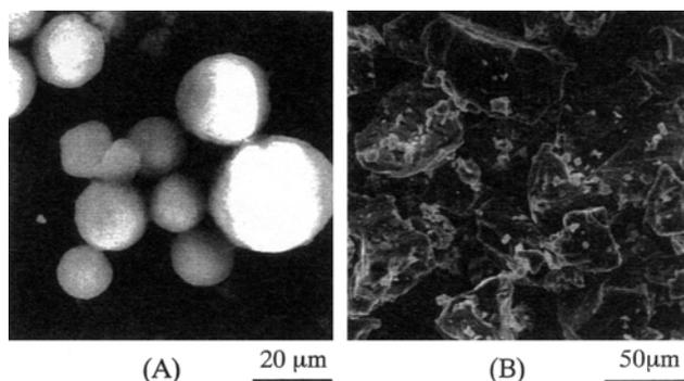
**Fig. 1.** SEM images of hydroxyapatite powder (A) and Ti powder (B).
