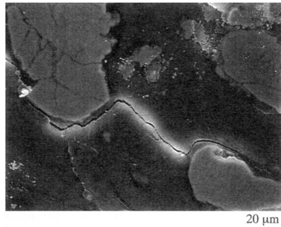
**Fig. 6.** SEM image of crack propagation in a hydroxyapatite/20 vol% Ti composite prepared by the PECS technique at 900°C.
