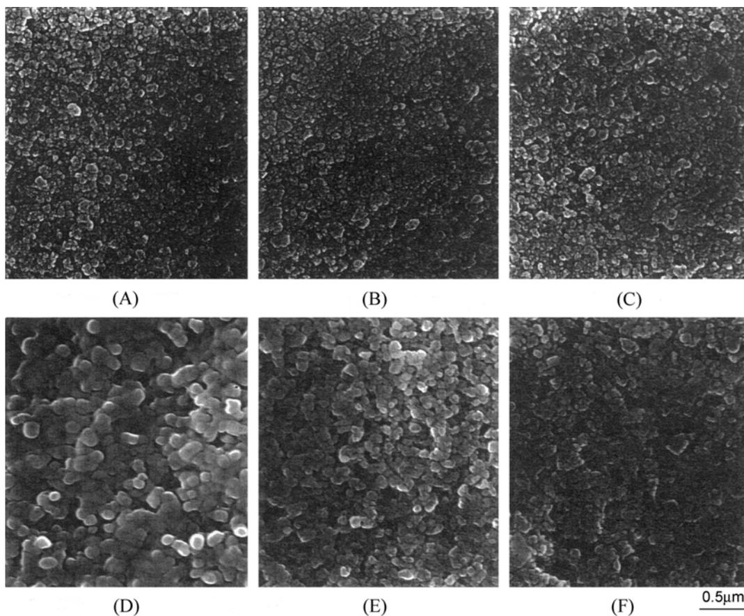
**Fig. 4.** SEM images of hydroxyapatite/Ti composites prepared by hot-pressing and PECS at 800-1000°C. (A) hot-pressed at 800°C (B) hot-pressed at 900°C (C) hot-pressed at 1000°C. (D) PECS at 800°C (E) PECS at 900°C (F) PECS at 1000°C. Bar shows 500 nm.
