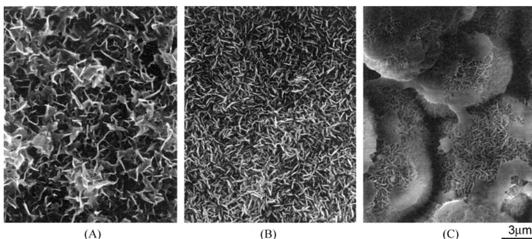
**Fig. 7.** SEM images of the precipitation on the surface of monolithic hydroxyapatite (A), hydroxyapatite/20 vol% Ti composite prepared by the PECS technique at 900°C (B) and hydroxyapatite/20 vol% Ti composite prepared by the hot-pressing technique at 900°C (C) after immersion in SBF solution at 36.5°C for 14 days.
