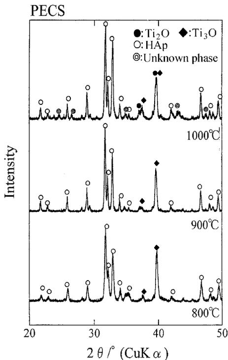
**Fig. 3.** XRD patterns of hydroxyapatite/20 vol% Ti composites prepared by a PECS process at 800-1000°C.
