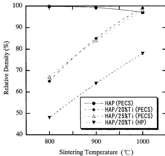
**Fig. 5.** Variations of the density with sintering temperature for hydroxyapatite/Ti composites prepared by hot-pressing (HP) and PECS techniques.
