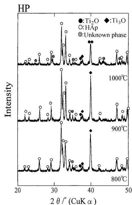
**Fig. 2.** XRD patterns of hydroxyapatite/20 vol% Ti composites hot-pressed at 800–1000°C.
