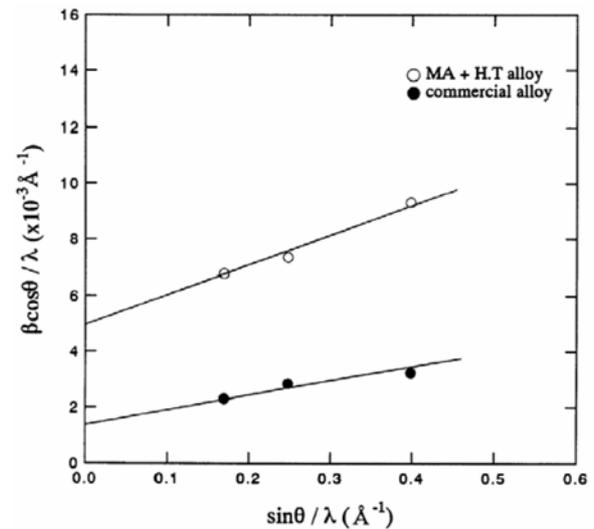
Fig. 6. Hall plot for the samples shown in Fig. 5.
