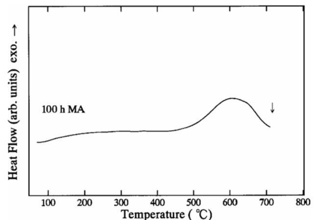
**Fig. 3.** DSC spectrum for  $\text{Mo}_{33}\text{Si}_{67}$  powders mechanically alloyed for 100 hours.
