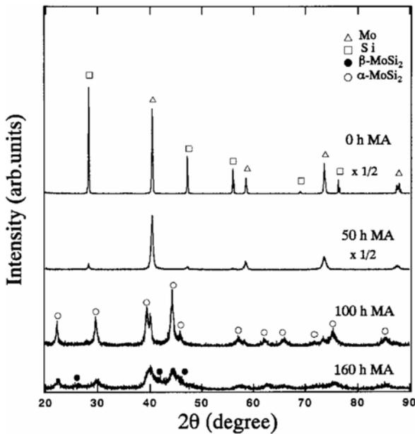
**Fig. 1.** X-ray diffraction patterns for  $\text{Mo}_{33}\text{Si}_{67}$  powders as a function of total MA time.
