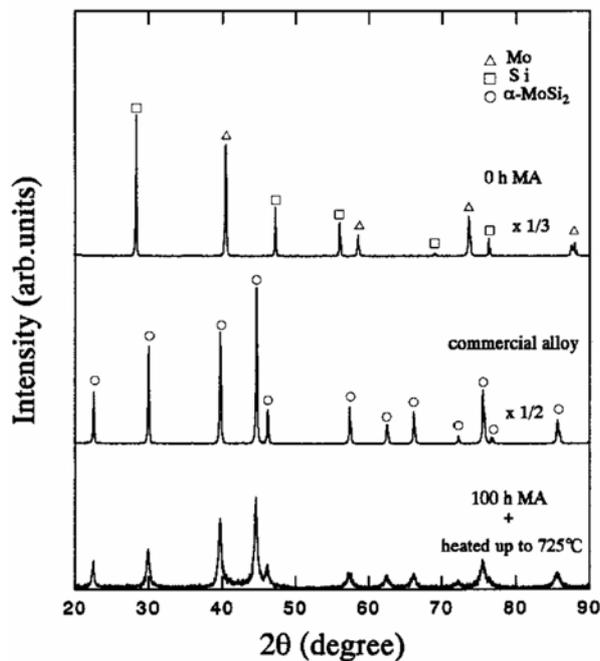
Fig. 5. X-ray diffraction patterns for the commercial MoSi<sub>2</sub> powders and 100 hours MA sample after heat treatment up to 725 °C.
