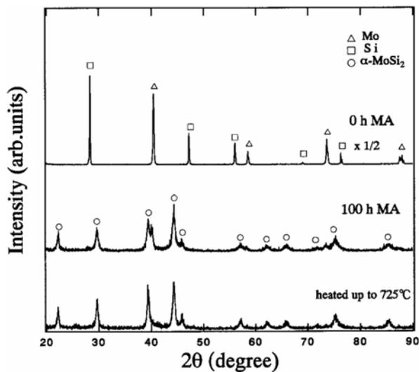
Fig. 4. Effect of heat treatment on the phase transformation for Mo<sub>33</sub>Si<sub>67</sub> powders mechanically alloyed for 100 hours.
