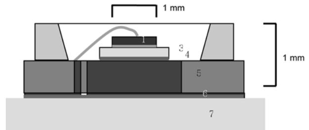
**Fig. 5.** Schematic diagram of working MLCMP. 1. vertically conductive LED (Epi-down) 2. Au-Sn eutectic solder 3. silicon submount (1.3\*1.6 mm<sup>2</sup>, 150 μm) 4. Ag-epoxy (2.5 W/m·K, 10 μm) 5. MLCMP 6. Pb-free solder (100 μm) 7. Metal PCB (75 μm Cu foil, 75 μm dielectric layer of 1.5 W/m·K on Aluminum).
