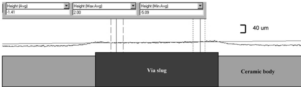
**Fig. 4.** Surface profile of the top surface of MLCMP. (The values in dialogue boxes were obtained within the intervals between vertical green lines. Diagram for illustration).
