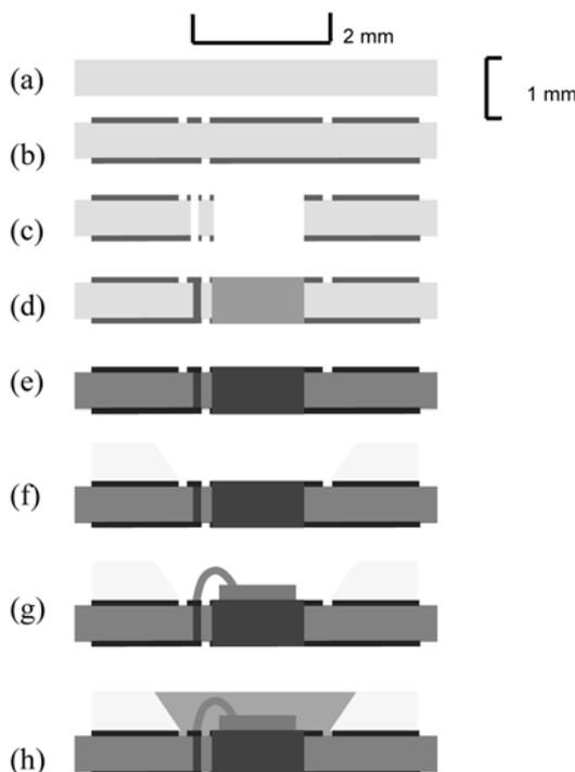
**Fig. 1.** Manufacturing process and structure of MLCMP. (a) green sheet lamination (b) pattern printing (c) punching (d) metal paste filling (e) firing (f) reflector attachment (g) chip mounting (h) encapsulation.
