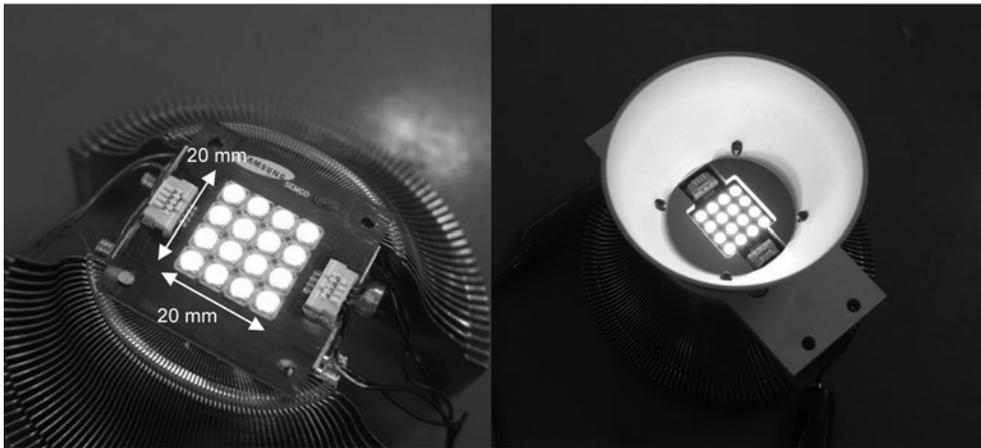
**Fig. 7.** Illumination module composed of 16 MLCMPs
