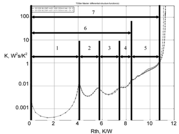
**Fig. 6.** Measured differential structure function showing thermal resistance of individual components consisting the working MLCMP. 1. Au-Sn eutectic solder 2. silicone submount 3. Ag-epoxy 4. via slug (MLCMP) 5. solder, PCB 6. junction to case 7. junction to board.
