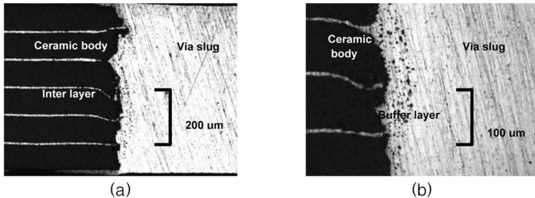
**Fig. 2.** Cross-section view of the ceramic body and via slug interface, showing. (a) wrinkle of the IL (b) interstratified layer from the BL.
