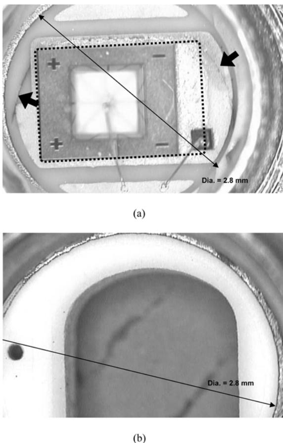
**Fig. 3.** Photographs showing the vicinity of the via slug after thermal shock tests. (a) in the case of a square via slug without a BL and IL, where the dashed line shows the via slug and bold arrows indicate cracks (b) in the case of a semi circular via slug with a BL and IL. No occurrence of cracks (the via slug was etched out for the examination).
