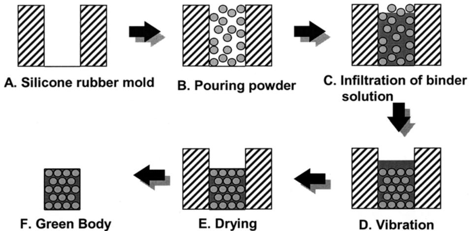
Fig. 3. Schematic illustrating pressureless powder packing (PLPP) forming method.
