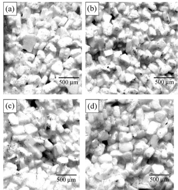
Fig. 12. Structures of PLPP specimens fired at 1150°C-2hr by PLPP method as a function of cullet content (x3); (a) 10 wt.%, (b) 20 wt.%, (c) 30 wt.% and (d) 40 wt.%.
