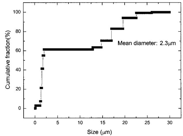
Fig. 8. Particle size distribution of cullet after attrition milling at 500 rpm=0.5 hr.
