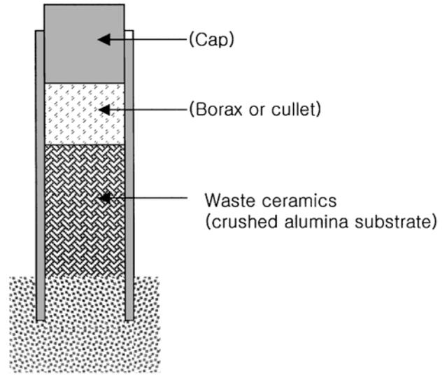
Fig. 2. Schematic illustrating of infiltration device.
