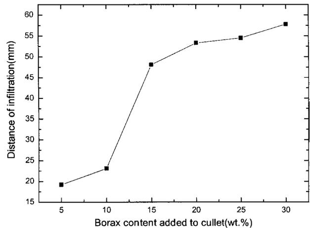
Fig. 11. Distance of flux infiltration as a function of borax contents added to cullet at 1150°C-2hr.
