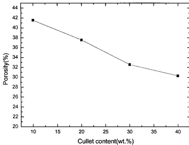
**Fig. 13.** Porosity of Pressureless Powder Packing (PLPP) specimens fired at  $1150^\circ\text{C}$ -2hr as a function of cullet contents.
