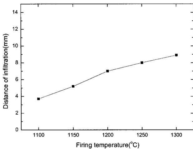
Fig. 10. Distance of infiltration of cullet as a function of firing temperature.
