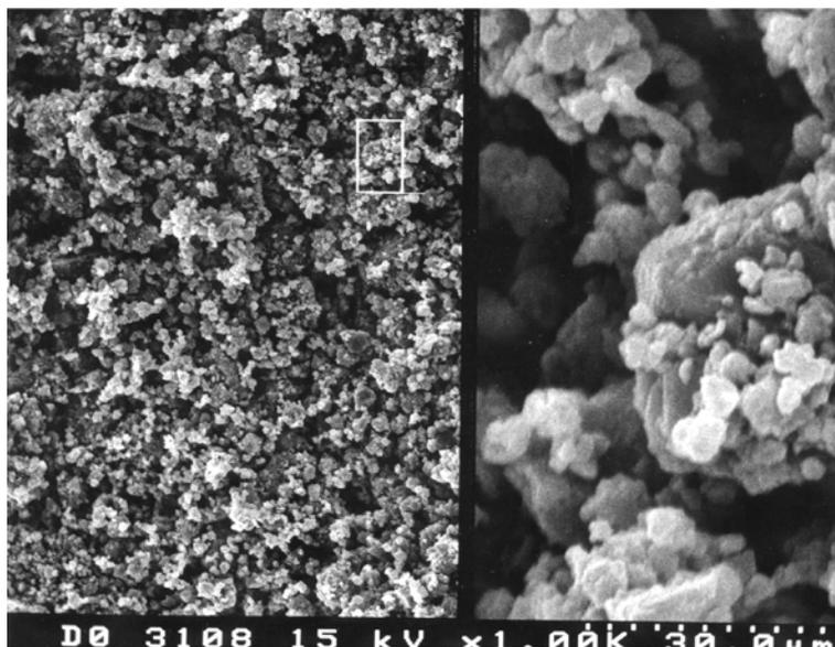
Fig. 7. SEM photograph alumina powder after attrition milling at 800 rpm-10 hr (<25 mesh).
