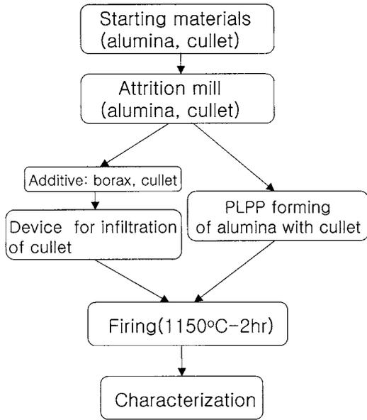
Fig. 1. Flow chart of overall process.
