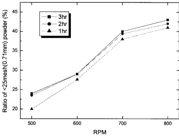
Fig. 5. Ratio of powder smaller than 25 mesh to total powder as a function of rpm and milling time.
