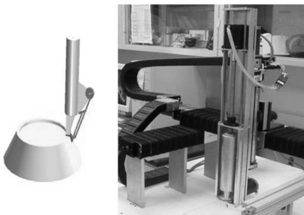
Fig. 1. CC machine (340\*380\*210mm) with the movable side trowel for fabricating complex 3D part.
