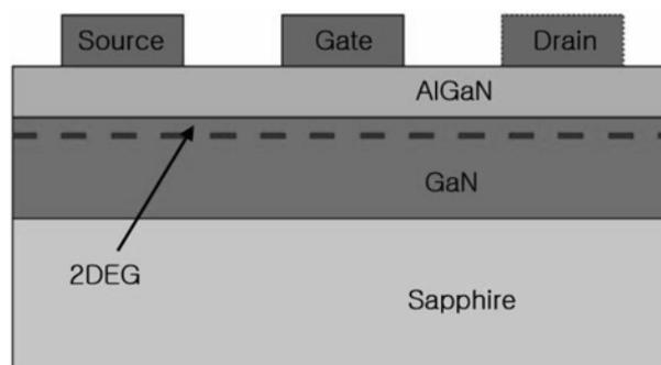
**Fig. 1.** Schematic Diagram of AlGa<sub>0.3</sub>N/GaN HEMT.
