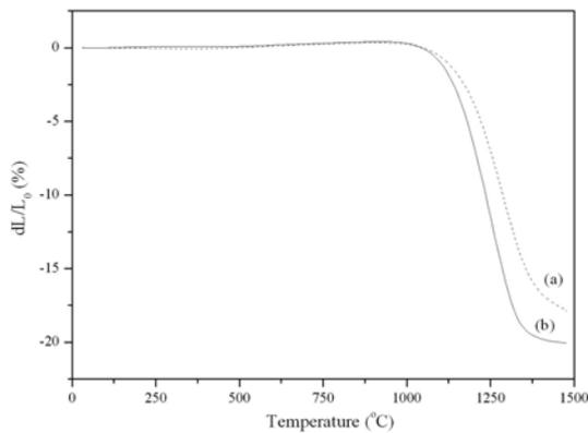
**Fig. 4.** The densification curves of Y-TZP powders without (a) and with (b) a boehmite coating.
