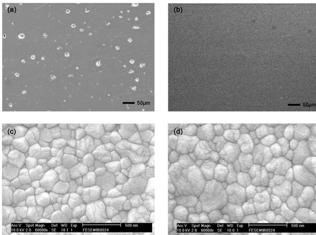
**Fig. 5.** The final microstructures of the samples without (a) (c) and with (b) (d) boehmite coating after sintering at 1350°C.
