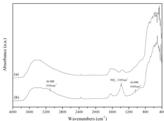
**Fig. 1.** FTIR spectra of Y-TZP powders before (a) and after (b) coating with boehmite.
