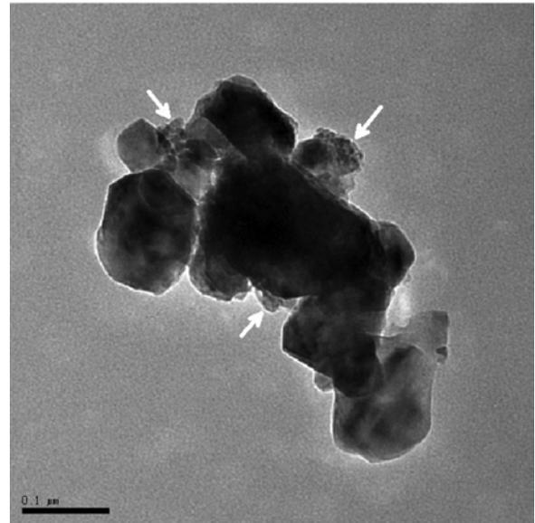
**Fig. 2.** TEM micrograph of Y-TZP powder coated with boehmite (the arrows: boehmite).
