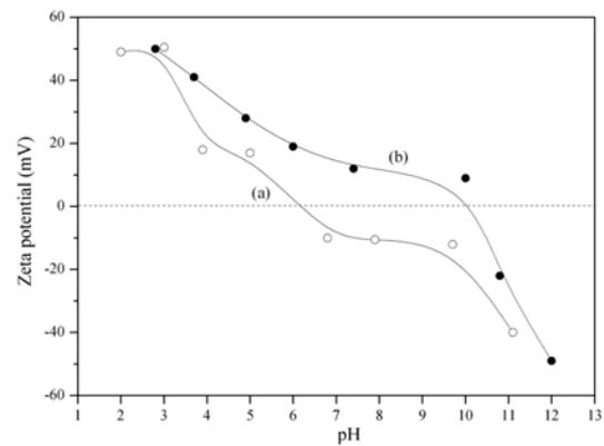
**Fig. 3.** Zeta potential as a function of pH for the Y-TZP powders without (a) and with (b) boehmite coating.
