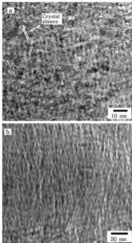
**Fig. 4.** TEM images for one of the carbon nanofilaments deposited at (a) 850 and (b) 950°C.
