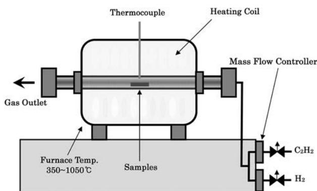
**Fig. 2.** Schematic diagram of the thermal chemical vapor deposition system for the carbon nanofilaments deposition.
