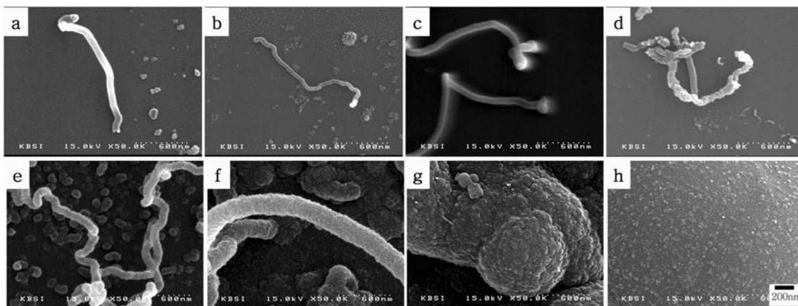
**Fig. 6.** High magnification FESEM images of the substrate surfaces deposited carbon nanofilaments at (a) 350, (b) 450, (c) 550, (d) 650, (e) 750, (f) 850, (g) 950 and (h) 1050°C.
