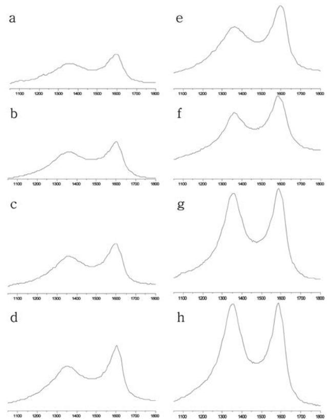
**Fig. 5.** Raman spectra of the substrate surfaces deposited carbon nanofilaments at (a) 350, (b) 450, (c) 550, (d) 650, (e) 750, (f) 850, (g) 950 and (h) 1050°C.
