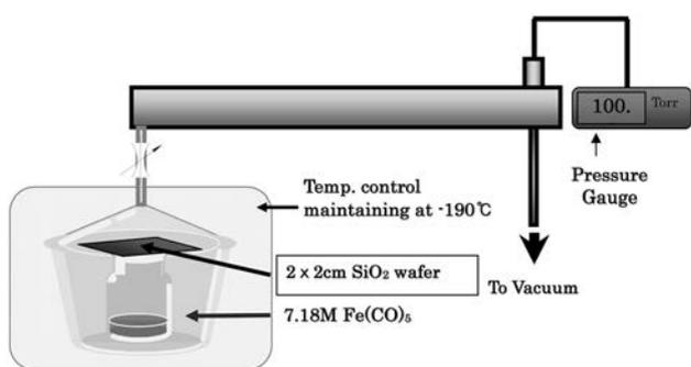
**Fig. 1.** Schematic diagram of vacuum-sublimation process for  $\text{Fe}(\text{CO})_5$  deposition on the  $\text{SiO}_2$  substrate.
