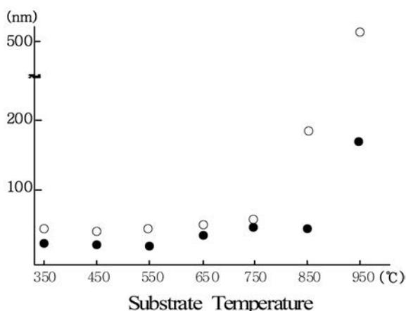
**Fig. 7.** Variations of the diameter (open circles) of carbon nanofilaments and the grain sizes of Fe metal catalyst particles (black circles) as a function of the substrate temperature.
