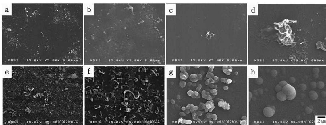
**Fig. 3.** FESEM images of the substrate surfaces deposited carbon nanofilaments at (a) 350, (b) 450, (c) 550, (d) 650, (e) 750, (f) 850, (g) 950 and (h) 1050°C.
