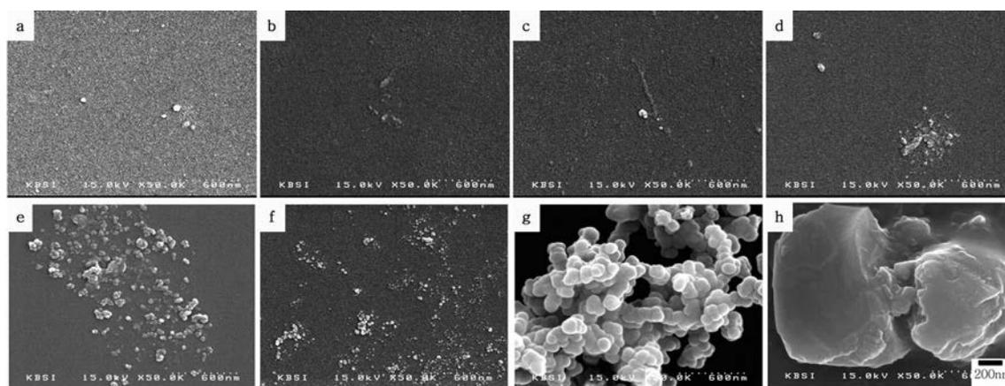
**Fig. 8.** FESEM images of the substrate deposited Fe metal catalyst nanograins after heating for 10 minutes in a vacuum at (a) 350, (b) 450, (c) 550, (d) 650, (e) 750, (f) 850, (g) 950 and (h) 1050°C
