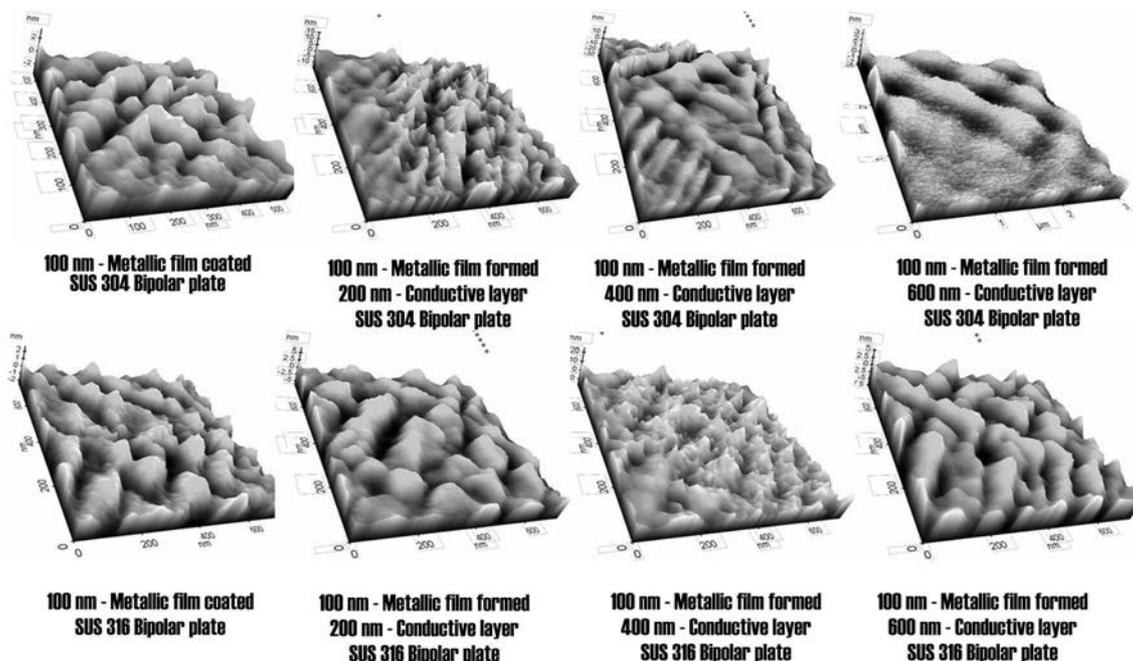
**Fig. 2.** AFM images of conductive film and metallic film coated-bipolar plates.
