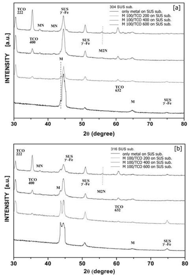
**Fig. 1.** (a) XRD patterns of metallic film [M: 100 nm] and conductive film [TCO: 200-600 nm] on stainless steel 304 plates. (b) XRD patterns of metallic film [M: 100 nm] and conductive film [TCO: 200-600 nm] on stainless steel 316 plates.
