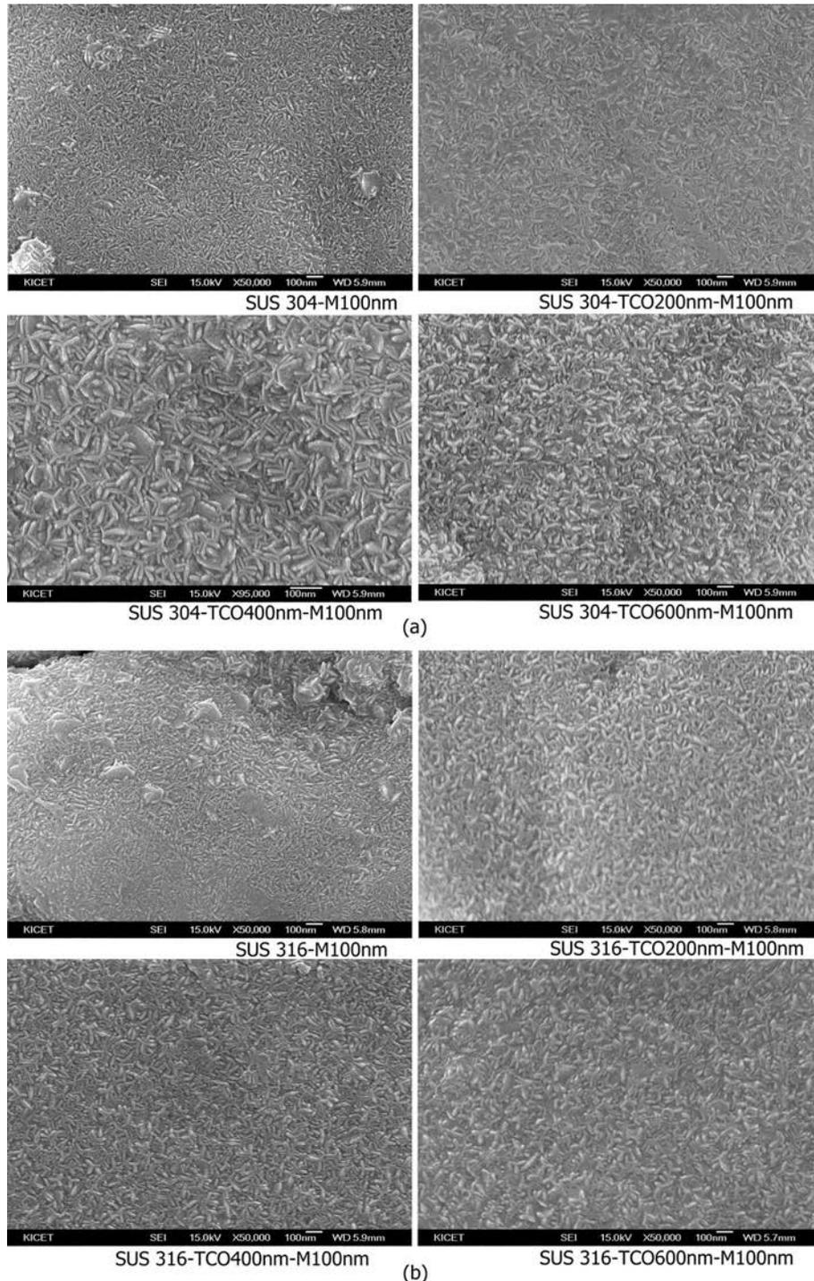
**Fig. 3.** (a), (b) FE-SEM images of metallic film [M] and conductive film [TCO] coated-SUS 304, 316 plates.
