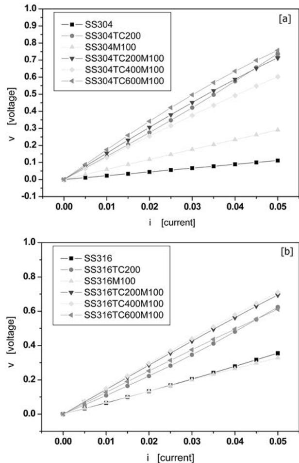
Fig. 4. (a), (b) I-V characteristics of metallic film [M: 100 nm] conductive film [TC: 200-600 nm] coated-SUS plates.
