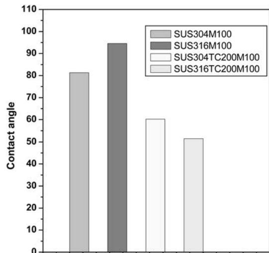
Fig. 5. Contact angles of metallic film [M: 100 nm] conductive film [TC: 200 nm] coated-SUS plates.
