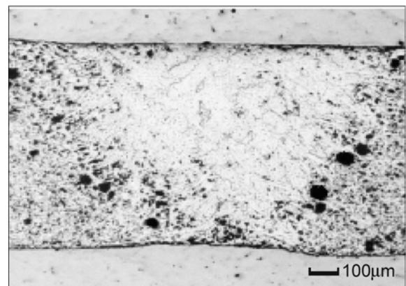
(b) cw welded seam
