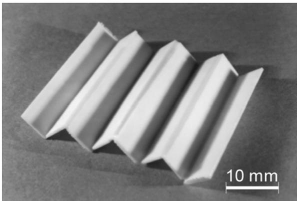
Fig. 6. Laser beam welded wave structure.
