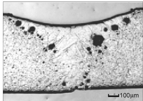
(a) pm welded seam
