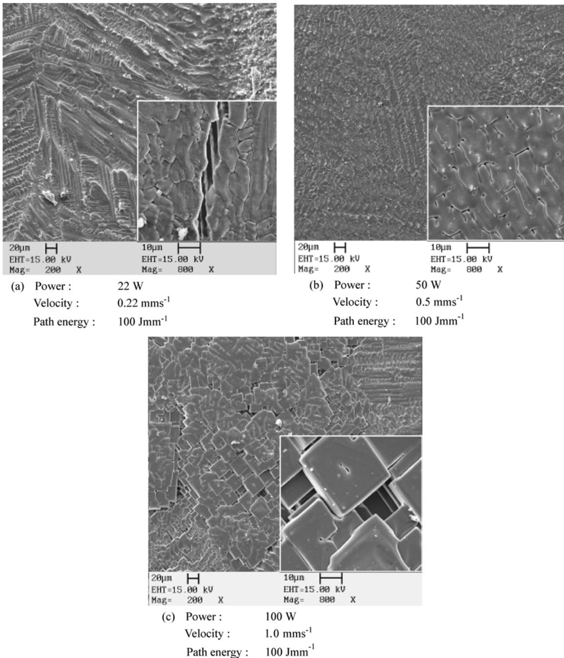
**Fig. 4.** Surface morphology at constant path energy and varying ratio of power and velocity.
