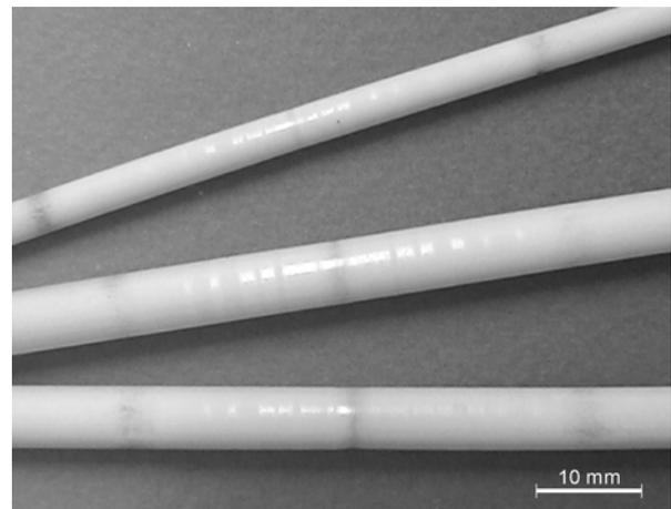
Fig. 8. Laser beam welded tubes.
