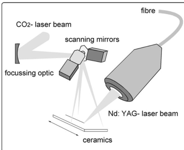
Fig. 1. Experimental setup used for laser welding of ceramics.
