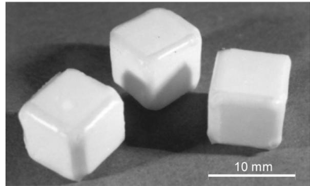
Fig. 7. Laser beam welded hollow cubes.
