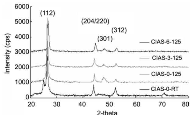
**Fig. 2.** XRD spectra of CIAS films with different Al contents and deposition temperatures.
