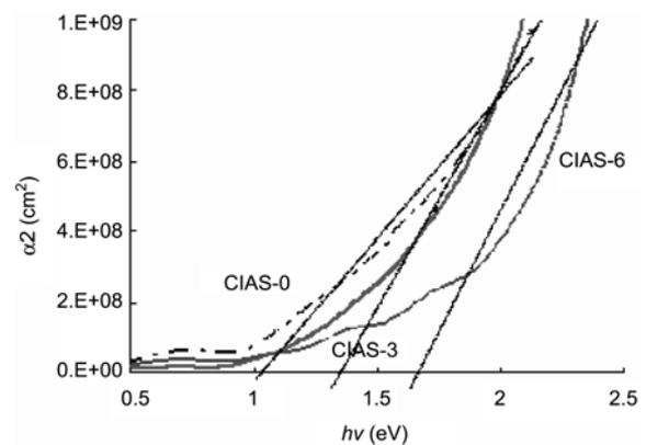
Fig. 5. Energy band gap of CIAS films deposited at 125 °C.
