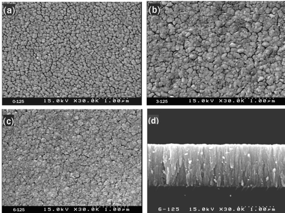
Fig. 3. Scanning electron micrographs of CIAS films deposited at 125 °C (a) CIAS-0 (b) CIAS-3 (c) CIAS-6 (d) cross section of CIAS-6.
