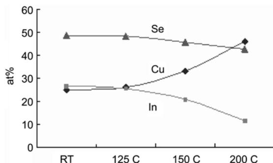
**Fig. 1.** EDX analysis of CIS films at different deposition temperatures.
