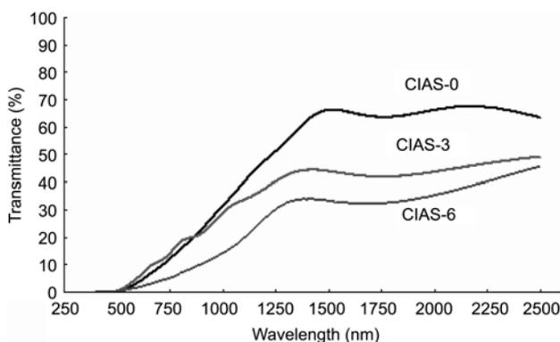
Fig. 4. Transmittance spectra of CIAS films deposited at 125 °C.
