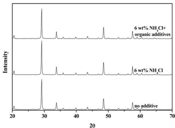
**Fig. 4.** XRD spectra of the phosphor particles prepared by spray pyrolysis.
