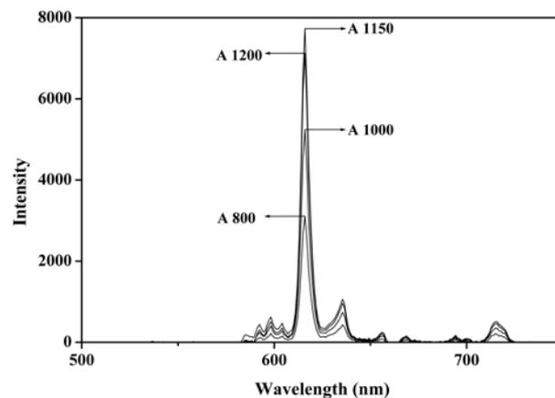
**Fig. 6.** Photoluminescence spectra of the phosphor particles post-treated at various temperatures. (A: post-treatment temperature in  $^\circ\text{C}$ )
