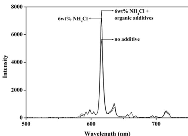
**Fig. 5.** Photoluminescence spectra of the phosphor particles prepared by spray pyrolysis.
