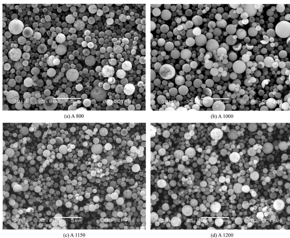
**Fig. 3.** SEM micrographs of the post-treated phosphor particles obtained from the spray solution with organic additives and the  $\text{NH}_4\text{Cl}$  flux. (A: post-treatment temperature in °C)
