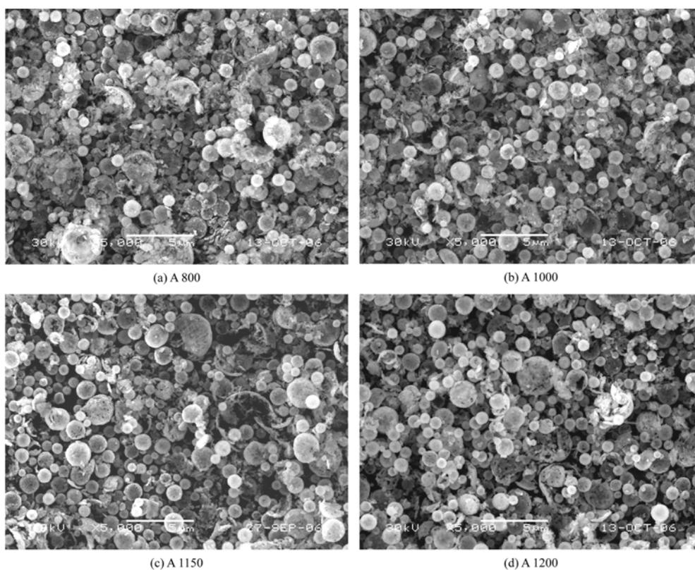
**Fig. 2.** SEM micrographs of the post-treated phosphor particles obtained from the spray solution with  $\text{NH}_4\text{Cl}$  flux. (A: post-treatment temperature in °C)
