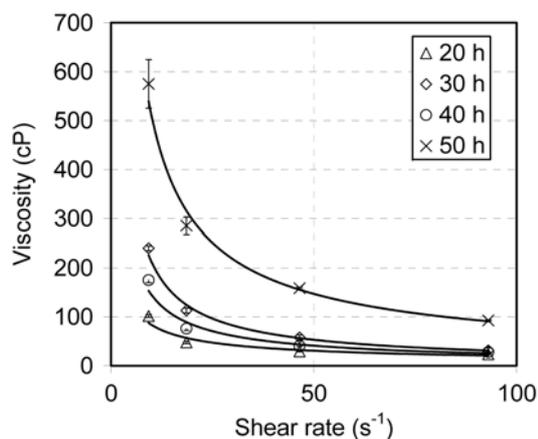
**Fig. 3.** Viscosity versus shear rate of various suspensions prepared using different ball milling times. Solid lines are fitted to power law equations (see text) indicating the shear thinning behavior of PZT aqueous suspensions.
