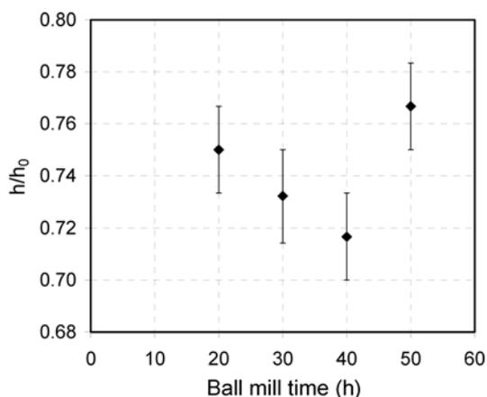
**Fig. 2.** Effects of ball milling time on sedimentation height ( $h/h_0$ ) of PZT aqueous suspensions.
