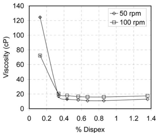
**Fig. 4.** Deflocculation curve of a 60 wt% solids loading PZT aqueous suspension ball milled for 30 h.
