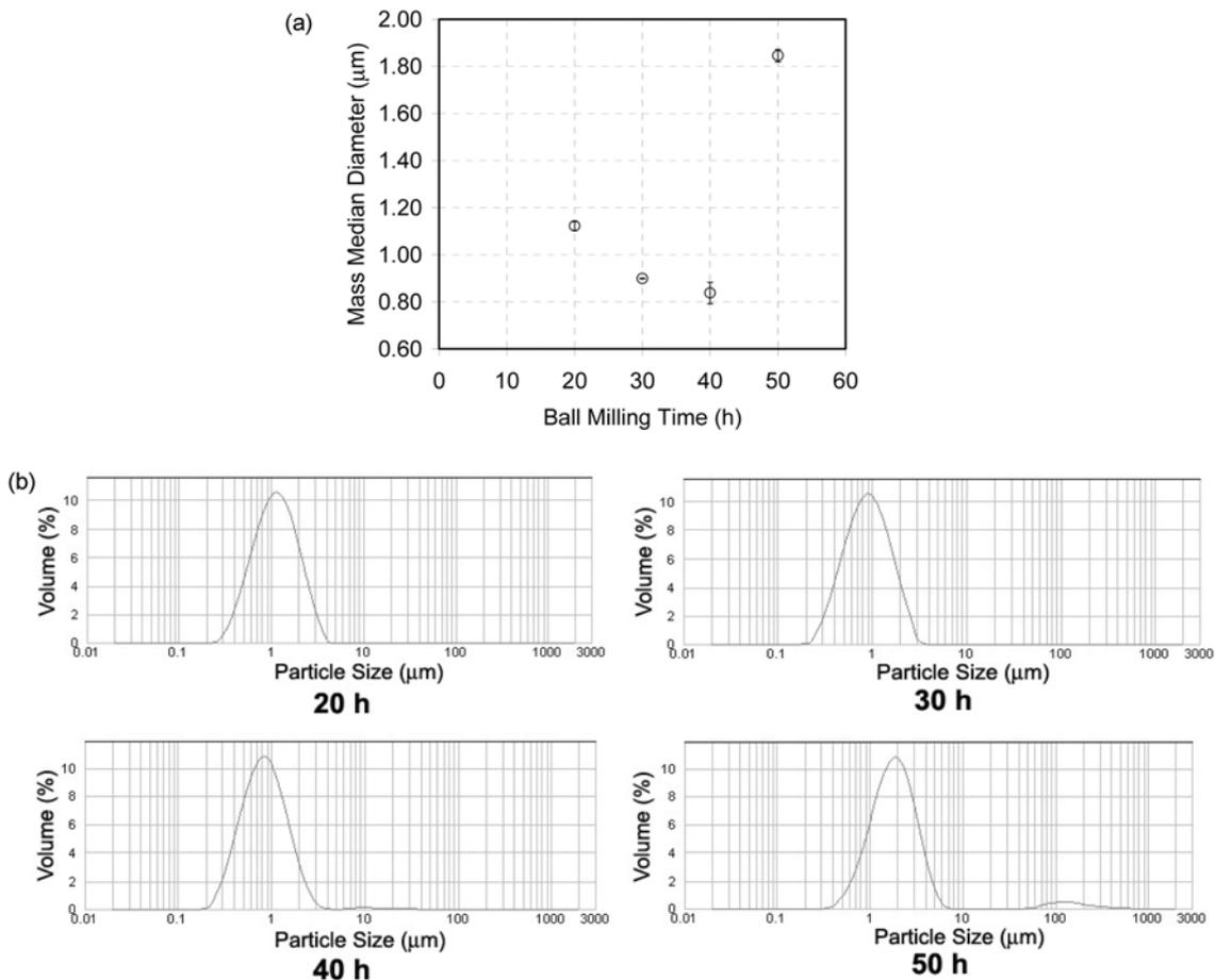
**Fig. 1.** (a) Average particle size for various ball milling times. (b) Particle size distribution of PZT for various ball milling times shown under the plots.
