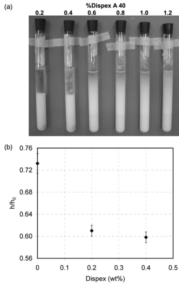
**Fig. 5.** (a) Precipitation behaviors of suspensions prepared with various Dispex A40 concentrations and (b)  $h/h_0$  ratios of completely precipitated suspensions.
