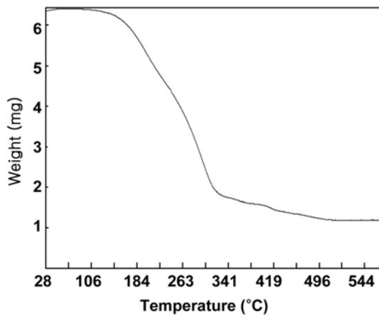
Fig. 3. TGA curve of the BIT solution used in this study.
