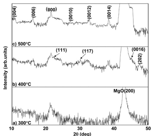
**Fig. 1.** XRD  $\theta$ - $2\theta$  scans of BIT films on MgO(100) substrates pyrolyzed at various temperatures, followed by final annealing at 750 °C.
