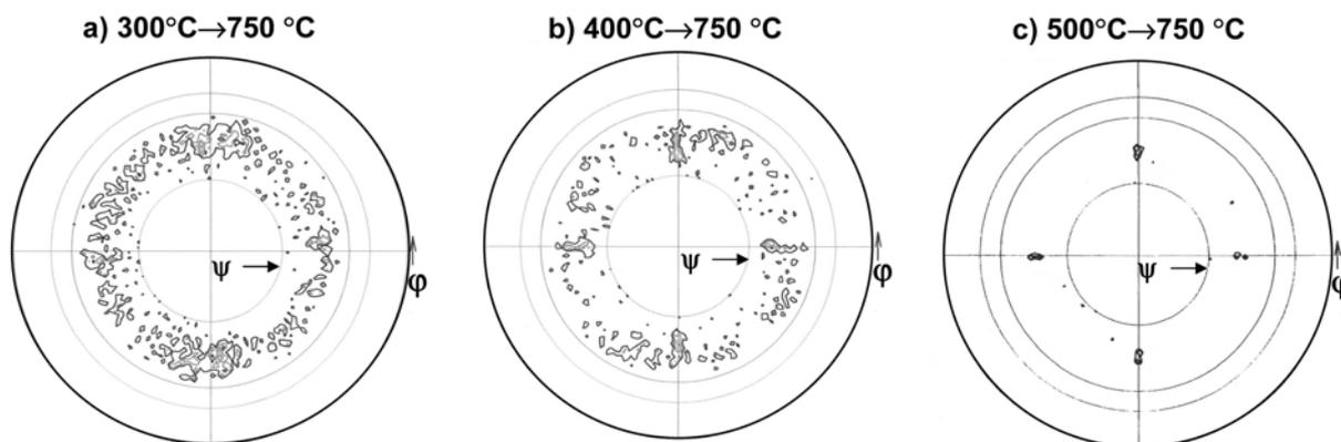
**Fig. 2.** X-ray pole-figures of BIT films pyrolyzed at various temperatures, followed by final annealing at 750 °C.
