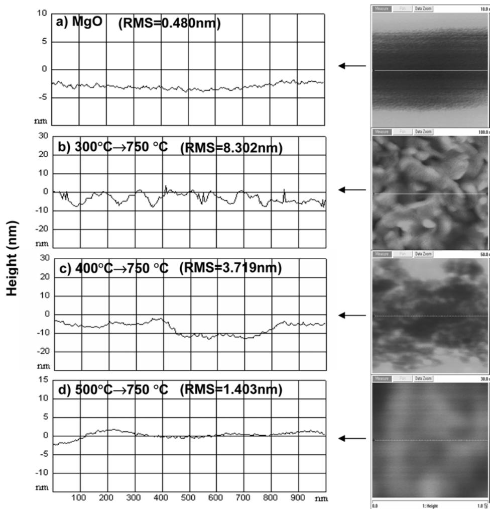
**Fig. 5.** SPM top-view images ( $1 \mu\text{m} \times 1 \mu\text{m}$ ) and surface roughness profiles of BIT films pyrolyzed at various temperatures, followed by final annealing at  $750^\circ\text{C}$ .
