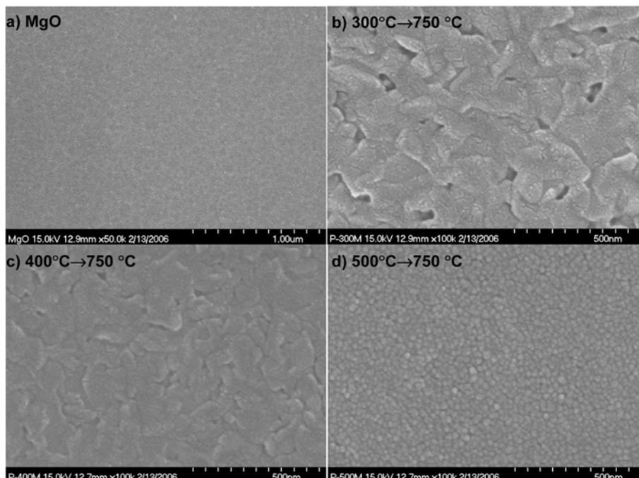
Fig. 4. FE-SEM images of BIT films pyrolyzed at various temperatures, followed by final annealing at  $750^\circ\text{C}$ .
