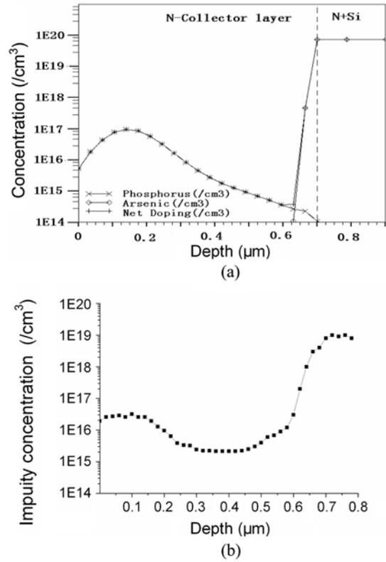
**Fig. 2.** (a) The simulated dopant profile; (b) The measured dopant profile by SRP.
