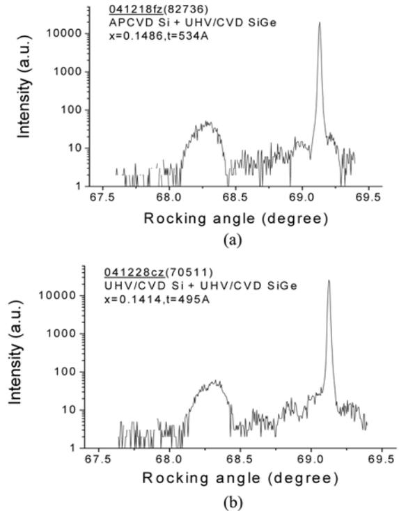
**Fig. 3.** The XRD rocking curves of (a) the SiGe on an N<sup>-</sup> collector by APCVD; (b) the SiGe on an N<sup>-</sup> collector by UHV/CVD i-Si epitaxy and ion implantation.
