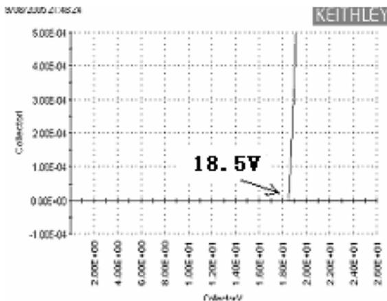
Fig. 6. Reverse BC junction I-V plot of the SiGeHBT with an N<sup>-</sup> collector grown by APCVD.
