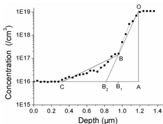
**Fig. 1.** The dopant profile in an N<sup>-</sup>collector layer grown by APCVD.
