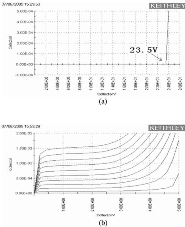
Fig. 5. Characteristics of the SiGeHBT with an N<sup>-</sup>collector by UHV/CVD i-Si epitaxy and ion implantation doping (a) reverse BC junction I-V plot; (b) output characteristics.
