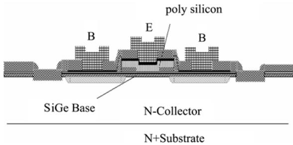
Fig. 4. The structure of the SiGeHBT.
