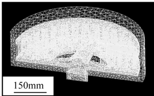
Fig. 3. Surface mesh of disk brake.
