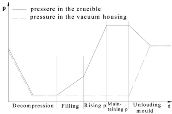
Fig. 1. pressure curve of adjustable vacuum pressure casting method.
