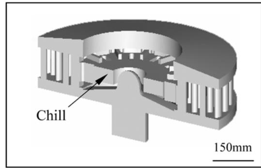
Fig. 8. Improved 3D-model of disk brake.
