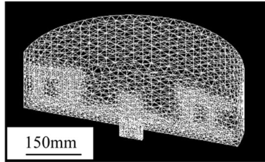
Fig. 4. Body mesh of disk brake.
