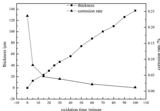
Fig. 1. Variation of thickness and corrosion rate of MAO coating on ZL205 with oxidation time.
