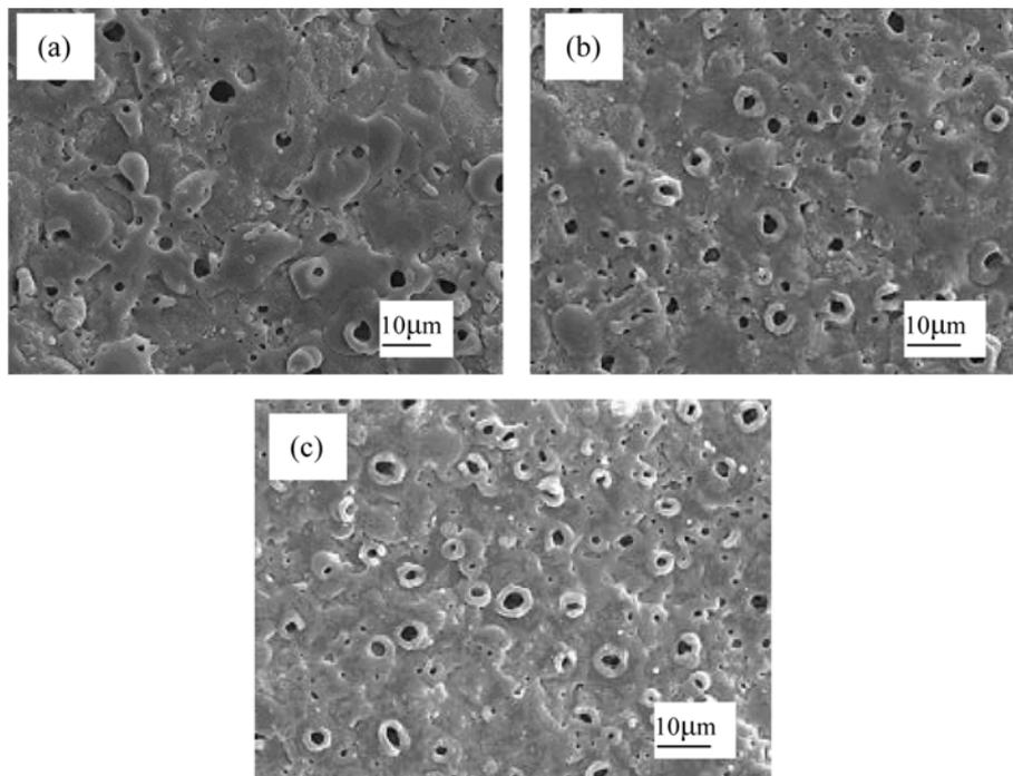
**Fig. 4.** Surface morphologies of MAO ceramic coatings on ZL205 with different current densities. (a) 22.38 A/dm<sup>2</sup>; (b) 11.5 A/dm<sup>2</sup>; (c) 7.5 A/dm<sup>2</sup>.
