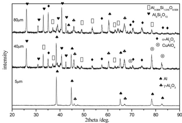
Fig. 5. XRD patterns of MAO coatings on ZL205 with different thickness.
