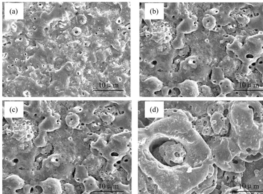
**Fig. 3.** Surface morphologies of MAO coatings on ZL205 with different oxidation times. (a) 5 minutes; (b) 20 minutes; (c) 60 minutes (d) 100 minutes
