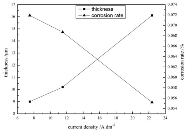
Fig. 2. Variation of thickness and corrosion rate of MAO coatings on ZL205 as a function of current density.
