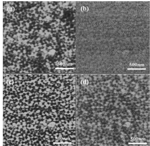
**Fig. 4.** Ferroelectric responses of nanotubes: (a) AFM image, (b) EFM image after applying  $V=0V$ , (c)  $V=+2V$  and (d)  $V=-2V$ .
