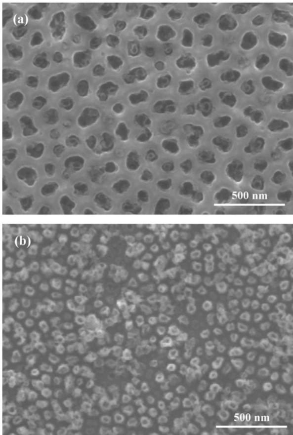
**Fig. 3.** SEM images of the PZT nanotube arrays: (a) top view of the nano porous alumina filled with PZT nanotubes, and (b) aligned PZT nanotube arrays by removal of part of the alumina.
