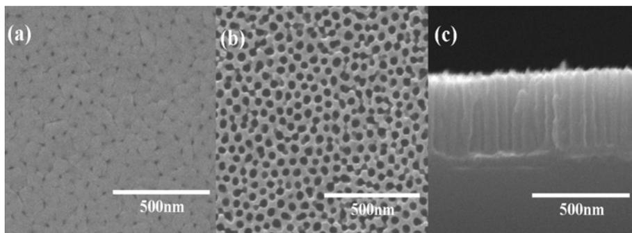
**Fig. 1.** SEM microphotographs of porous alumina after the second anodization and widening processes (a) view of the surface (after the second anodization) (b) view of the surface (after the widening process) and (c) cross sectional view.
