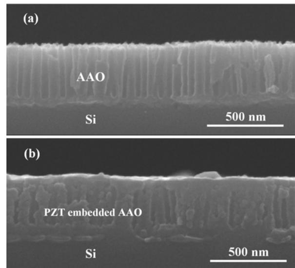
**Fig 2.** Cross sectional view of nanostructures for (a) as received alumina nano pores and (b) PZT embedded alumina nano pores.
