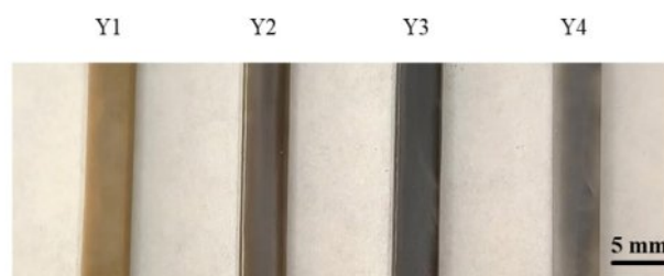
Fig. 10. Appearance of glass-ceramics with different B_2O_3 contents.
