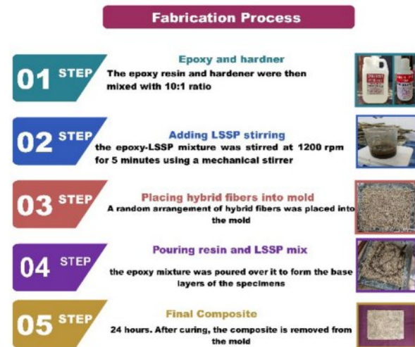
Fig. 3. Experimental process for the fabrication of composites.
