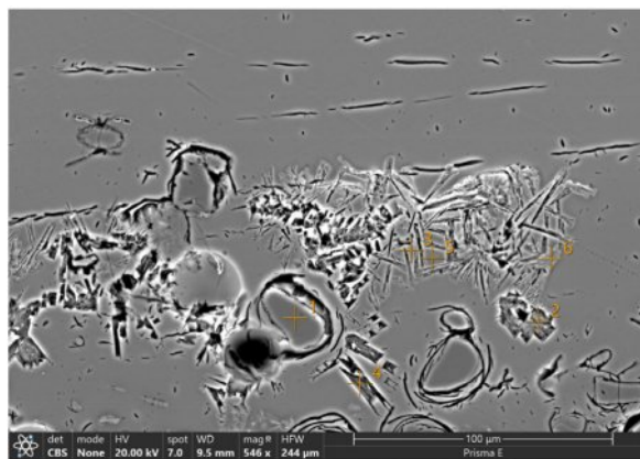
Fig. 8. Microstructure of the glaze-body interface in sample GFZ-2.
