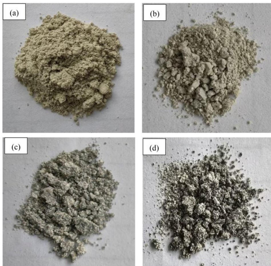
Fig. 5. Macroscopic morphology of SiC-ZrB 2 composite powders after 30-min oxidation at: (a) 800 °C, (b) 1000 °C, (c) 1200 °C, (d) 1500 °C.
