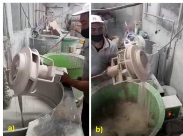
Fig. 2. Example of coating: a) Coating slurry to wax pattern, b) Coating stucco
