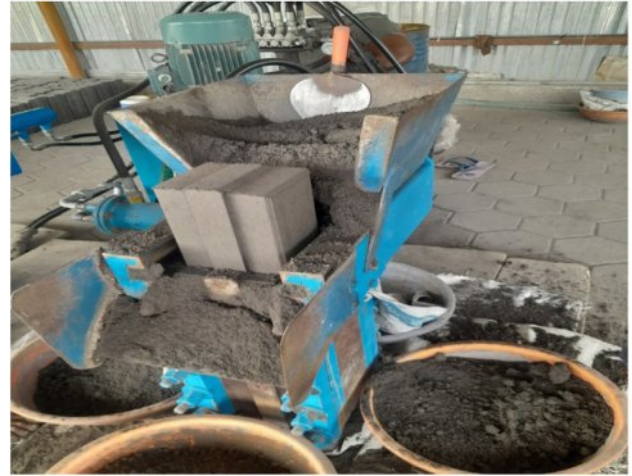
Fig. 3. Interlocking brick production in an industrial setup.
