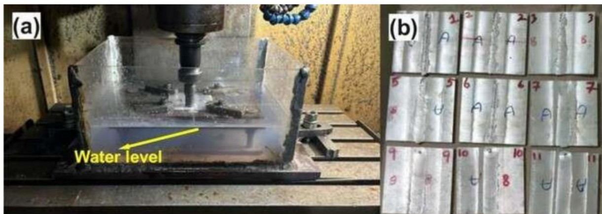
Fig. 4. (a) Experimental setup of underwater friction stir welding. (b) Welded samples.
