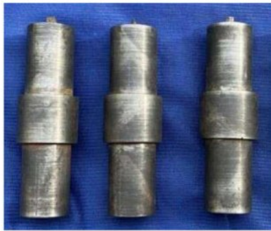
Fig. 3. Types of tool profiles for UFSW (a) square, (b) Cone, and (c) hexagon.
