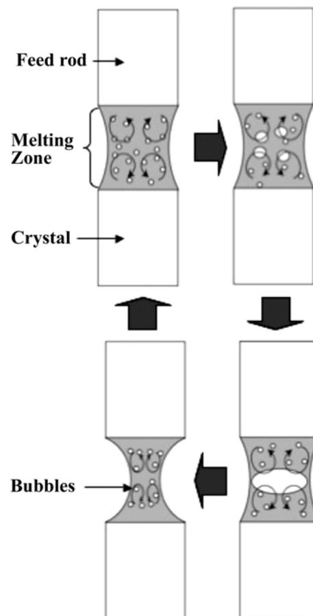
**Fig. 3.** Schematic illustration of the behavior of oxygen bubbles in the melt during conventional FZ growth.
