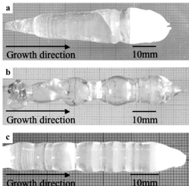
**Fig. 2.** Single crystals grown under various conditions; (a) sintered feed rod and an oxygen atmosphere, (b) unsintered feed rod and an oxygen atmosphere, (c) unsintered feed rod and a nitrogen atmosphere.
