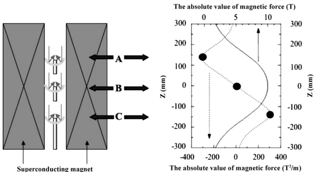
**Fig. 1.** Schematic of growth stage along direction of magnetic force; (A) high position, downward magnetic force is a maximum on an oxygen bubble (B) center of superconducting magnet, (C) low position, upward magnetic force is a maximum.
