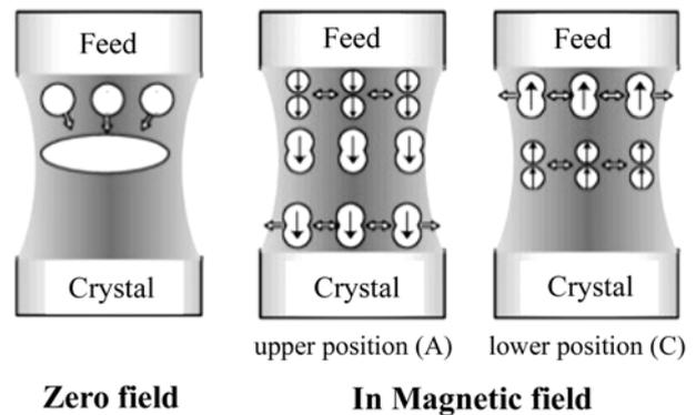
**Fig. 5.** Schematic illustration of behavior of bubbles in the melt without magnetic field (left), and under a magnetic field; high position (middle) and low position (right).
