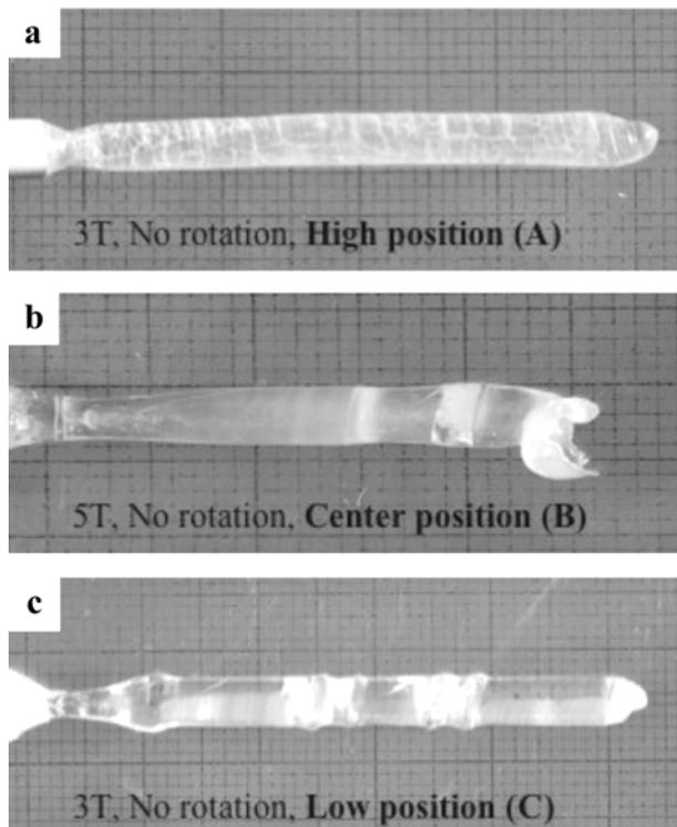
**Fig. 4.** Single crystals grown under magnetic field; (a) 3 T at the high position, and (b) 5 T at the center position, and (c) 3 T at the low position.
