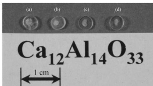
**Fig. 6.** Cross-section images of crystals grown at the low position under (a) 1 T, (b) 3 T, (c) 5 T, and (d) 8 T (left). This shows a reduction of bubble density with increasing magnetic fields (right).
