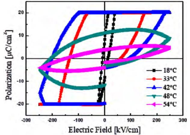
Fig. 6. Hysteresis loops of  $K(\text{Ta}_{0.6}\text{Nb}_{0.4})\text{O}_3$  thin films sintered at 750 °C.
