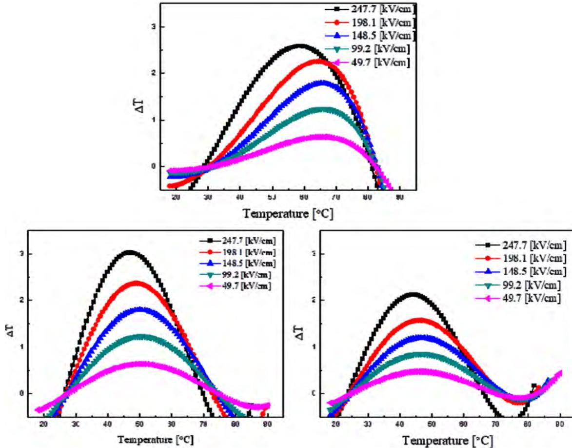
Fig. 8. Electrocaloric properties ( $\Delta T$ ) of  $K(\text{Ta}_{0.6}\text{Nb}_{0.4})\text{O}_3$  thin films with temperature changes.
