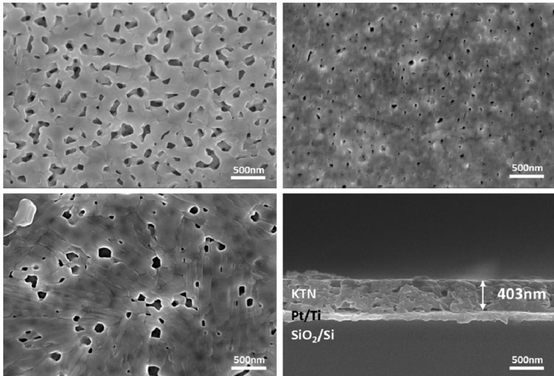
**Fig. 2.** Surface and cross-sectional microstructures of  $K(\text{Ta}_{0.6}\text{Nb}_{0.4})\text{O}_3$  thin films with the sintering temperatures; (a) surface, 700 °C, (b) surface, 750 °C, (c) surface, 800 °C and (d) cross-section, 750 °C.
