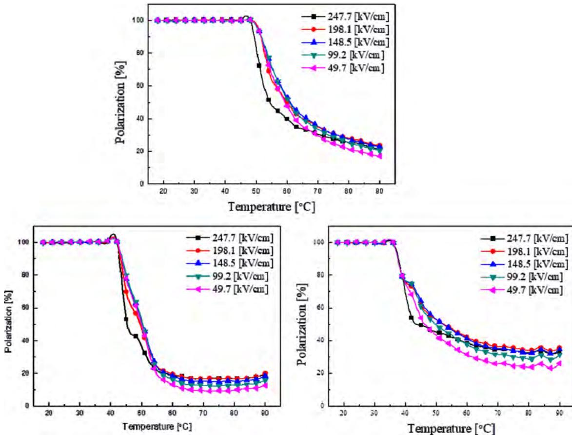
Fig. 7. Polarization of  $K(\text{Ta}_{0.6}\text{Nb}_{0.4})\text{O}_3$  thin film with temperature and voltage application.
