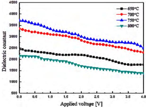
Fig. 5. Relative dielectric constant of  $K(\text{Ta}_{0.6}\text{Nb}_{0.4})\text{O}_3$  thin films with DC voltage applied.
