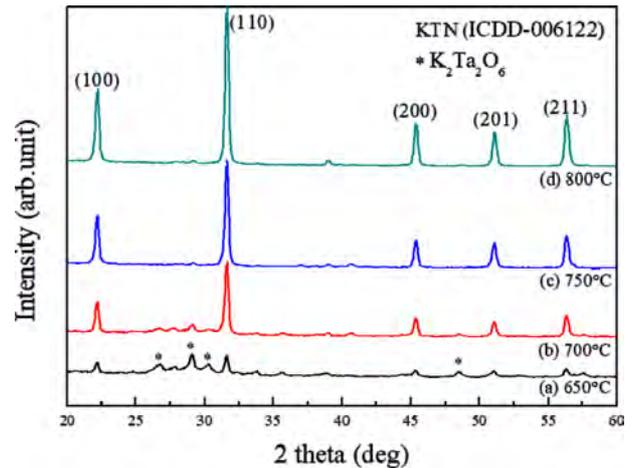
Fig. 1. X-ray diffraction patterns of  $K(\text{Ta}_{0.6}\text{Nb}_{0.4})\text{O}_3$  thin films according to the sintering temperature.
