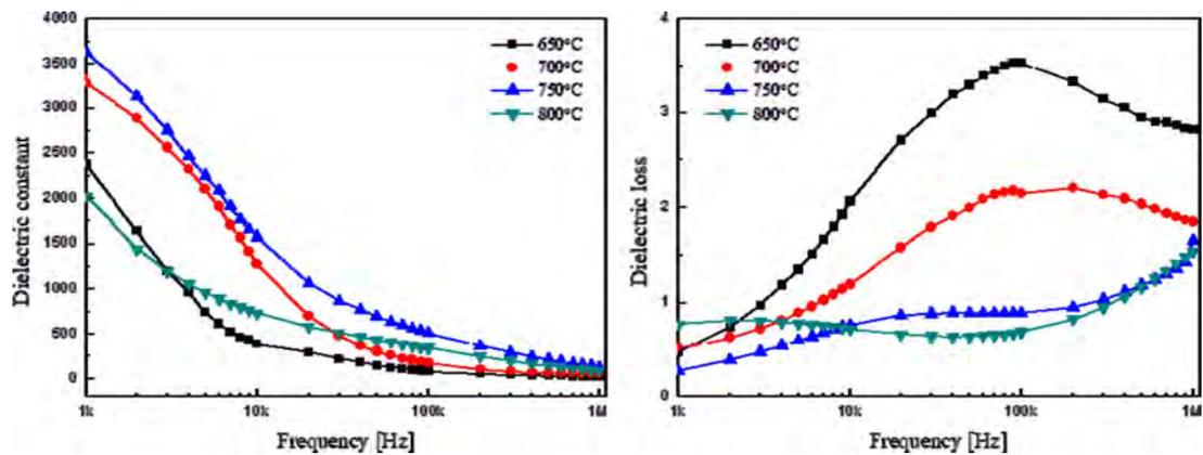
**Fig. 3.** Relative dielectric constant and dielectric loss of  $K(\text{Ta}_{0.6}\text{Nb}_{0.4})\text{O}_3$  thin films with the applied frequency.
