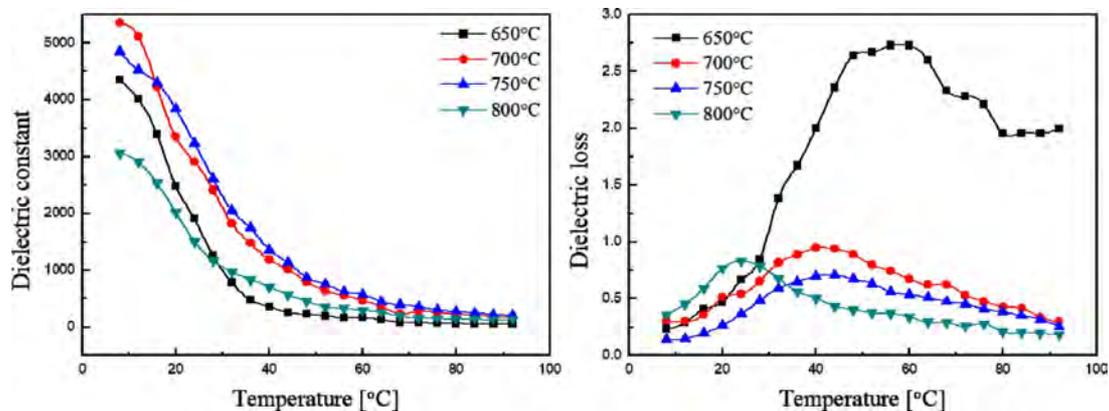
**Fig. 4.** Relative dielectric constant and dielectric loss of  $K(\text{Ta}_{0.6}\text{Nb}_{0.4})\text{O}_3$  thin films.
