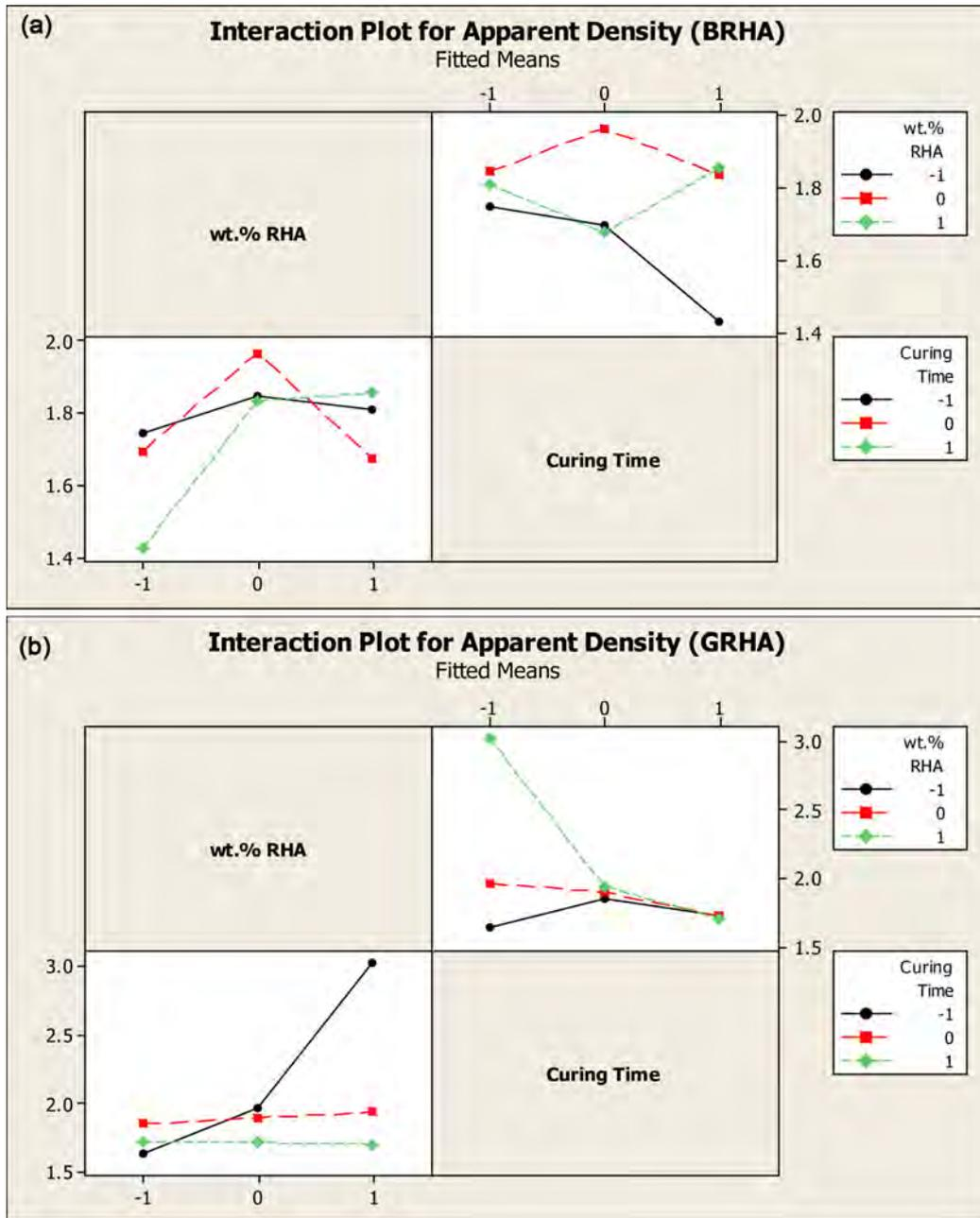
Fig. 9. (a) Interaction Plots for Apparent Density (BRHA). (b) Interaction Plots for Apparent Density (GRHA).
