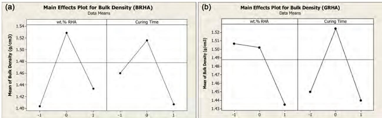
Fig. 10. (a) Main Effects Plot for Bulk Density (BRHA). (b) Main Effects Plot for Bulk Density (GRHA).
