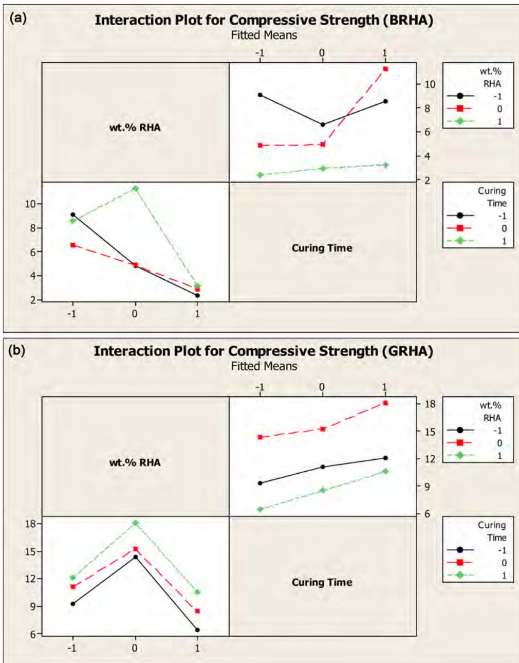
Fig. 5. (a) Interaction Plot for Compressive Strength (BRHA). (b) Interaction Plot for Compressive Strength (GRHA).
