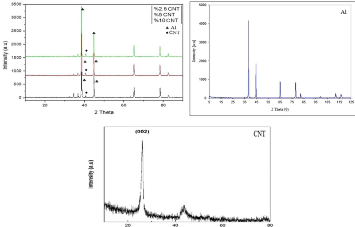
Fig. 6. XRD pattern of 2.5-7.5 % content MWCNTs particles in Al matrix, Aluminum and CNT.
