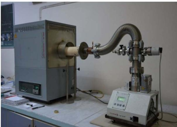
Fig. 1. Sintering process for horizontal pipe furnace system.
