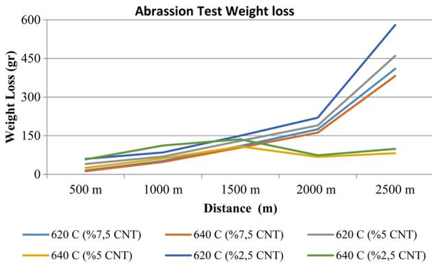
**Fig. 3.** Abrasion test results of the specimens in different temperatures and CNT ratios.
