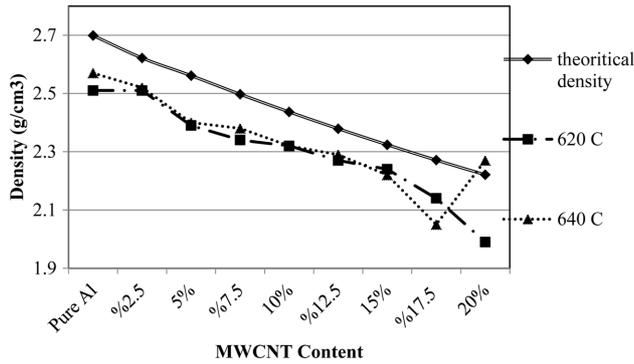
**Fig. 7.** Density at different % MWCNT content sintering temperatures.
