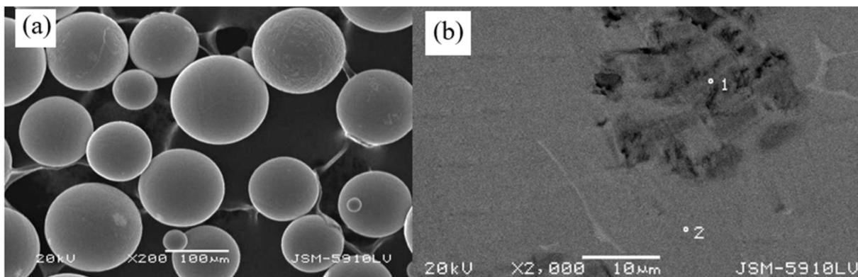
**Fig. 4.** The MWCNTs reinforced matrix Al SEM images of the composite material. (a): Spherical Al particulate, (b): 1. Al/MWCNT phase and 2. Al composite materials.
