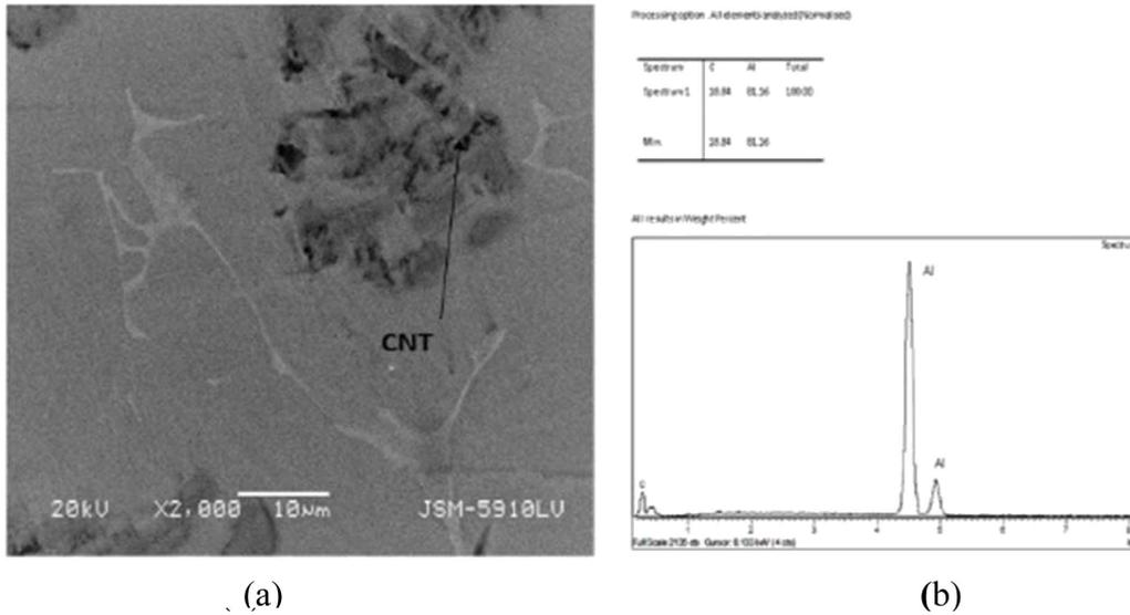
Fig. 5. The composite material's (7.5 % content Al/MWCNT) of (a) SEM image, (b) EDS analysis.
