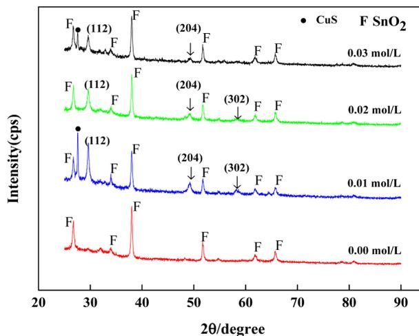
Fig. 3. XRD patterns of thin films prepared with different of  $\text{Na}_2\text{S}_2\text{O}_3 \cdot \text{H}_2\text{O}$  after sulfurization.
