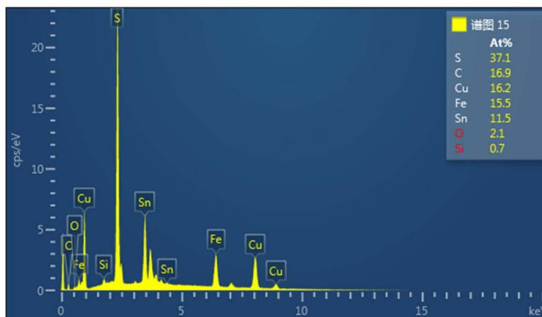
Fig. 5. EDS spectrum showing the elemental composition of synthetic CuFeS<sub>2</sub>.
