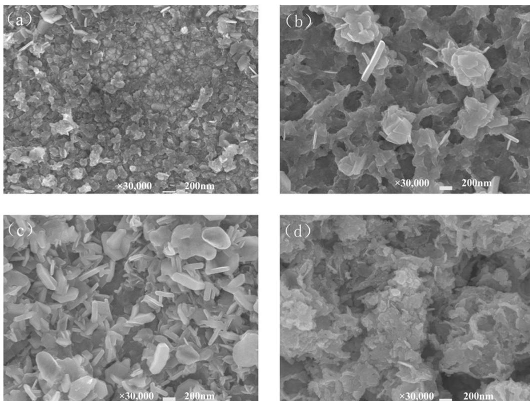
Fig. 4. Morphology of samples prepared by electrodeposition after sulfurization. (a) 0.00 M; (b) 0.01 M; (c) 0.02 M; (d) 0.03 M.
