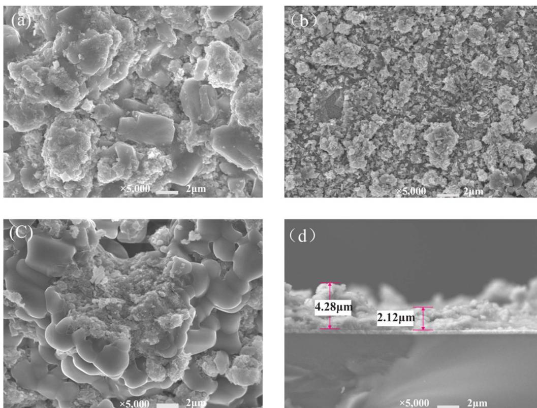
**Fig. 2.** Morphology of samples prepared by electrodeposition after sulfurization. (a) pH = 3; (b) pH = 4; (c) pH = 5; (d) Cross section of thin film.
