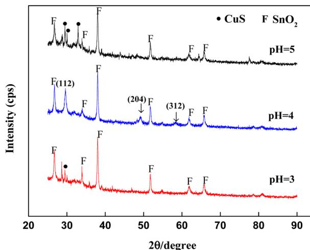
**Fig. 1.** XRD patterns of thin films prepared at pH 3-5 after sulfurization.
